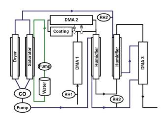
642 Figure 1. Schematic diagram of the coating-hygroscopicity tandem differential mobility analyzer. Here,
