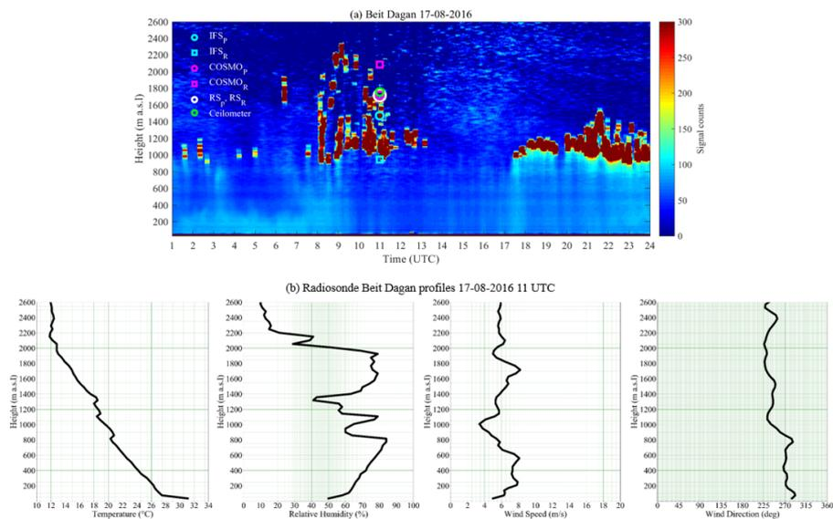
Fig.8 Ceilometer signal counts plot on August 17, 2016, including indications of the PBL heights at 11 UTC from the models (IFS<sub>R</sub>, IFS<sub>p</sub>, COSMO<sub>R</sub>, COSMO<sub>p</sub>), radiosonde (RS<sub>R</sub>, RS<sub>p</sub>) and ceilometer (a). The bottom panel presents the radiosonde profiles retrieved at 11 UTC on the same day (b).
