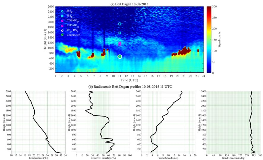
Fig.10 Ceilometer signal counts plot on August 10, 2015, including indications of the PBL heights at 11 UTC from the models (IFS<sub>R</sub>, IFS<sub>P</sub>, COSMO<sub>R</sub>, COSMO<sub>P</sub>), radiosonde (RS<sub>R</sub>, RS<sub>P</sub>) and ceilometer (a). The bottom panel presents the radiosonde profiles retrieved at 11 UTC on the same day (b).
