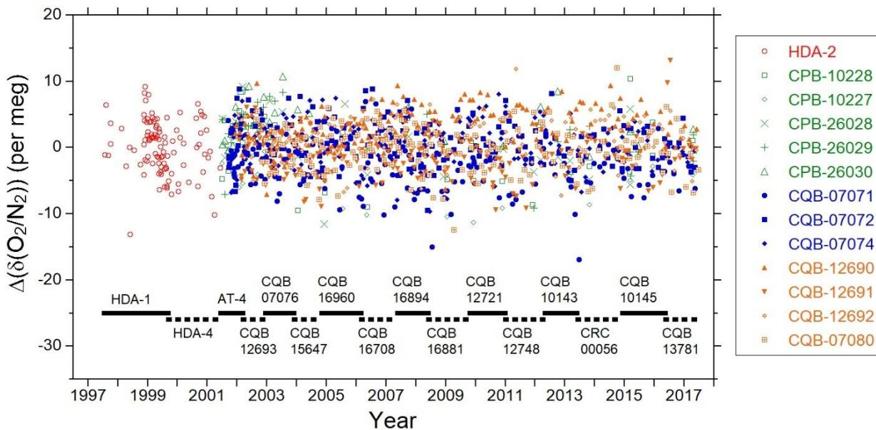
**Fig. 2.** Temporal changes in the O<sub>2</sub>/N<sub>2</sub> ratio of primary reference gases relative to the NIES O<sub>2</sub>/N<sub>2</sub> scale. The differences of the O<sub>2</sub>/N<sub>2</sub> ratio from the average are plotted for HDA-2 along with the differences of the O<sub>2</sub>/N<sub>2</sub> ratio from the initial values for the individual cylinders except HDA-2. Solid and broken horizontal bars in the lower part of the figure indicate the periods when
