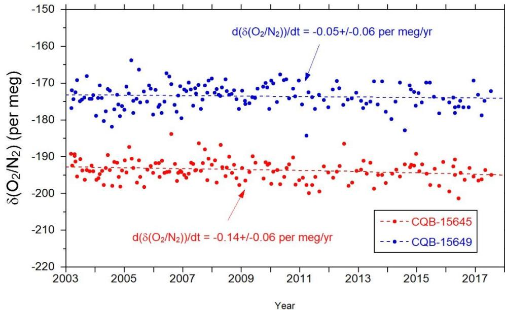
**Fig. 3.** Temporal changes in the  $\text{O}_2/\text{N}_2$  ratio of reference airs in two aluminum cylinders which are independent from the NIES primary reference gases, relative to the NIES  $\text{O}_2/\text{N}_2$  scale. The broken lines represent the linear regression lines.
