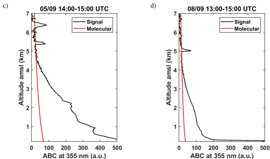
773 **Figure A2:** Apparent backscatter coefficient (black solid lines) profiles obtained from the ASL lidar in Henties Bay on:
