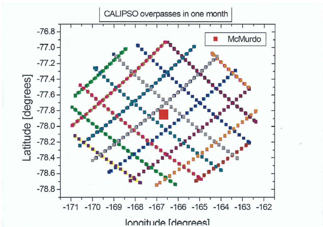
McMurdo. While CALIOP provides a resolution of 5 km ( when integration is required due to low signal-to-noise ratio up to 135 km !) the air mass sampled by the ground-based lidar extends to at most 100 m. (30 km \* 3 mrad field of view of the telescope).
