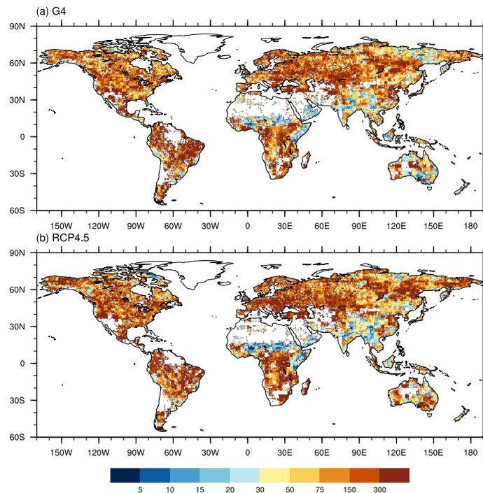
Figure 9: Multi-model ensemble range of return period for discharge that correspond with the 30-year return period in the historical simulation (1960-1999) under (a) G4 and (b) RCP4.5 scenarios, as the difference between maximum and minimum return periods. Grid cells in extremely dry regions, i.e.  $Q_m < 0.01$  mm/day and extreme high value of return period regions were masked out.
