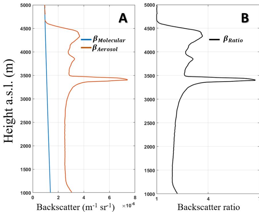
Figure 14 – (A)  $\beta_{Molecular}$  (blue line) and  $\beta_{Aerosol}$  (orange line). (B)  $\beta_{Ratio}$  (black line). All profiles were obtained from the 532 nm lidar signal
