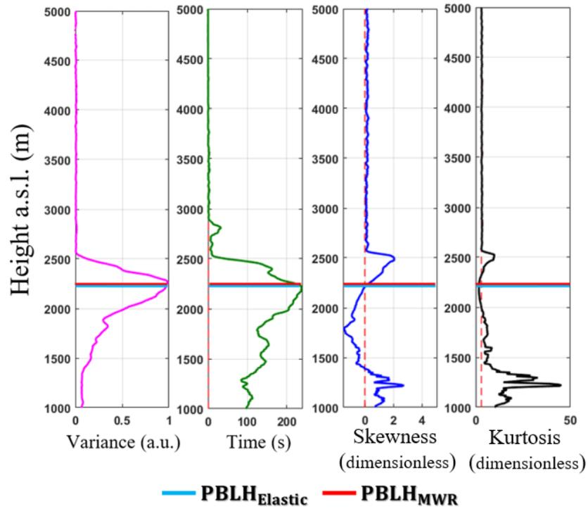
Figure 11 – Statistical moments obtained from elastic lidar data at 13 to 14 UTC - 19 May 2016. From left to right: variance [ $\sigma_{RCS'}^2$ ], integral time scale [ $\tau_{RCS'}$ ], skewness [ $S_{RCS'}$ ] and kurtosis [ $K_{RCS'}$ ].
