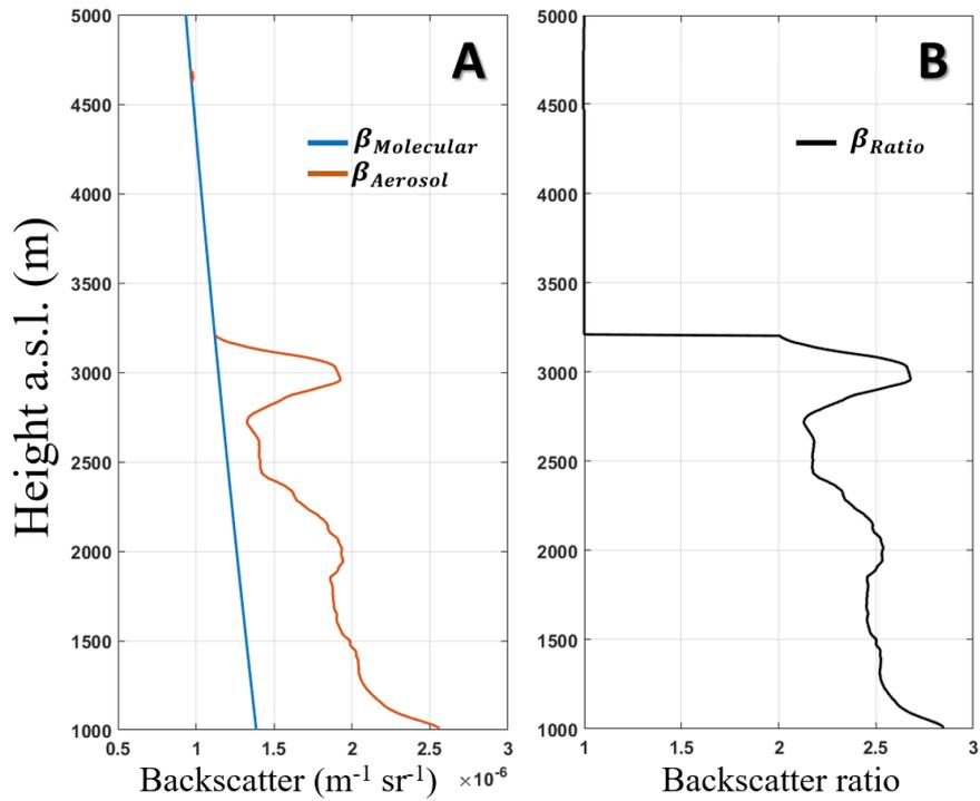
Figure 10 – (A)  $\beta_{Molecular}$  (blue line) and  $\beta_{Aerosol}$  (orange line). (B)  $\beta_{Ratio}$  (black line). All profiles were obtained from the 532 nm lidar signal
