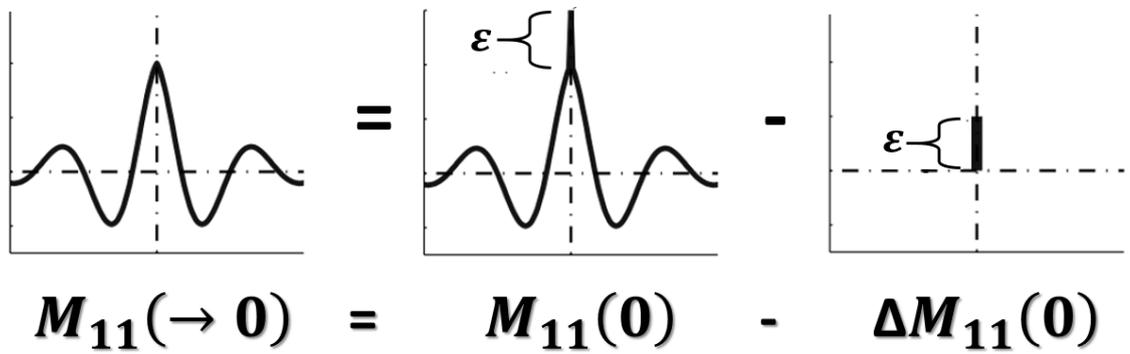
Figure 1 – Procedure to remove the errors of autocovariance functions.  $M_{11}(\rightarrow 0)$  – corrected autocovariance function errors;  $M_{11}(0)$  - autocovariance function without correction;  $\Delta M_{11}(0)$  - error of autocovariance function
