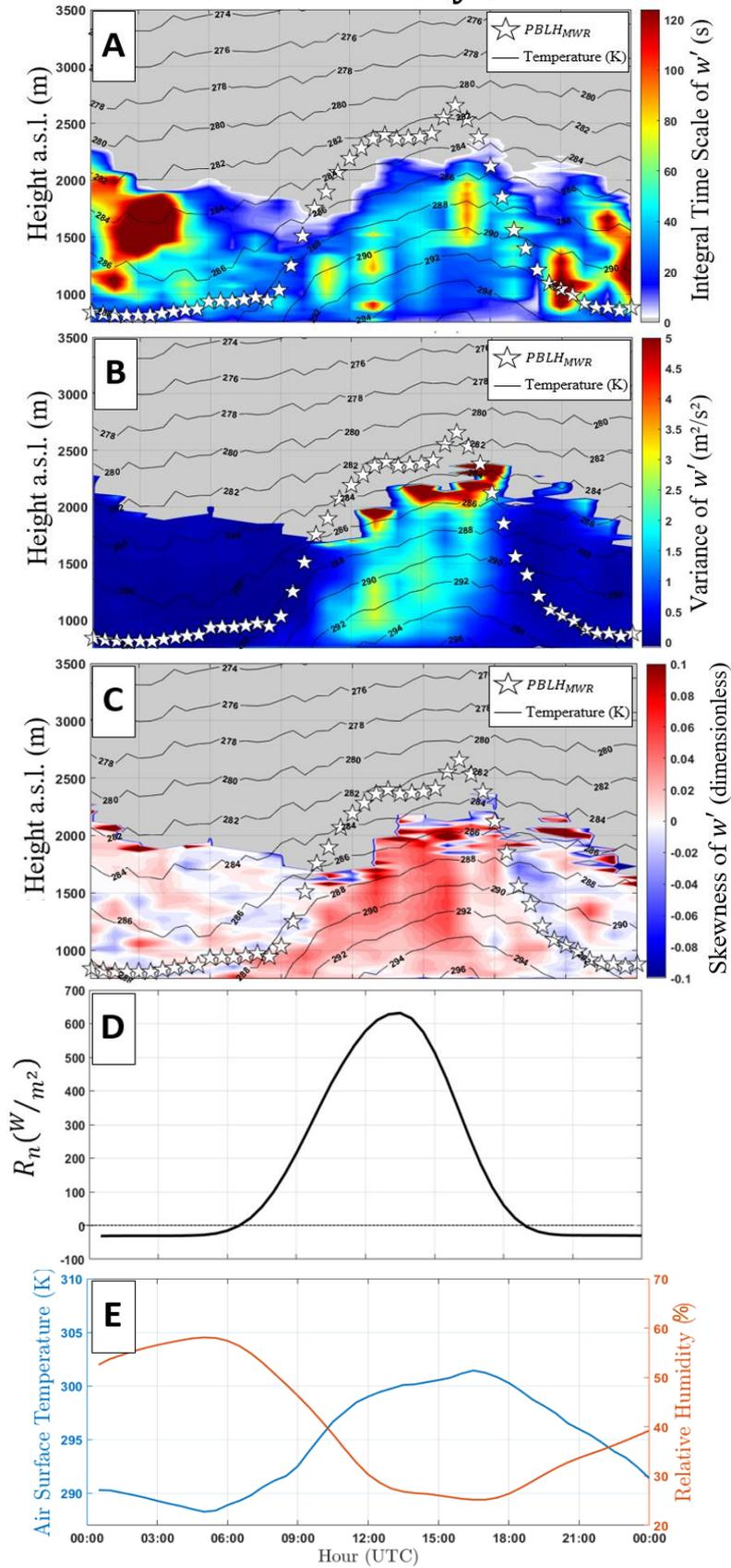
Figure 8 – A – integral time scale [ $\tau_{w'}$ ], B – variance [ $\sigma_{w'}^2$ ], C – skewness [ $S_{w'}$ ], D – net radiation [ $R_n$ ], E – Air surface temperature [blue line] and surface relative humidity [RH – orange line]. In A, B and C black lines and white stars represent air temperature and  $PBLH_{MWR}$ , respectively.
