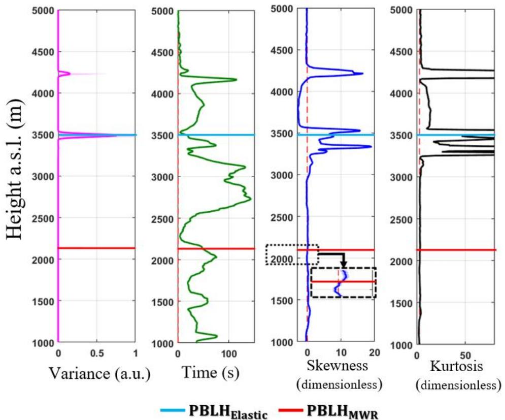
Figure 16 - Statistical moments obtained from elastic lidar data at 12 to 13 UTC - 08 July 2016. From left to right: variance [ $\sigma_{RCS'}^2$ ], integral time scale [ $\tau_{RCS'}$ ], skewness [ $S_{RCS'}$ ] and kurtosis [ $K_{RCS'}$ ].
