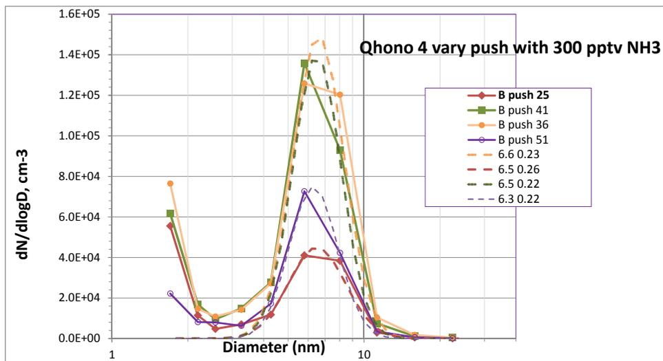
**Fig. 1.** Showing the effect of changing the total flow from the ammonia source, through an 1/8" OD tube.
