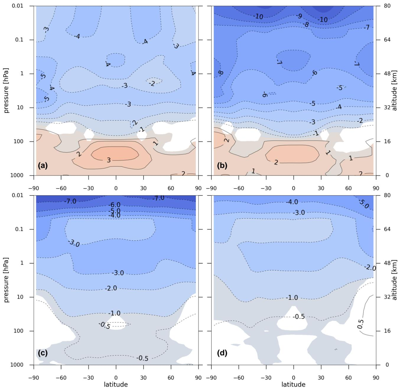
**Figure 4: Annual zonal mean temperature difference in K of future (2090–2099) minus near present (2000–2009) for REF (a) and SD (b), and difference SD – REF (c) and WD – REF (d) under future conditions (2090–2099). Coloured regions are significant at the 95% confidence level (calculated using a Student  $t$ -test). Colour interval is 1 K.**
