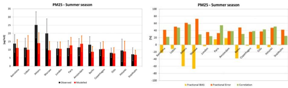
**Figure 4.** Evaluation of CAMx model performance for PM<sub>2.5</sub> at selected cities for July 1 to September 30, 2010. Left panel compares the observed (black) and modeled (red) seasonal mean concentrations. Bars show the corresponding observed (grey) and modeled (orange) standard deviation. Right panel shows the seasonal Fractional Bias (orange), Fractional Error (red) and Correlation (green) computed for each city.
