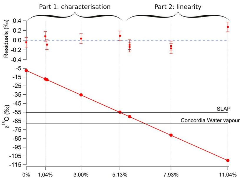
470 *Figure 6:* Isotopic composition measured by liquid injector in the Picarro L2140i for different samples
