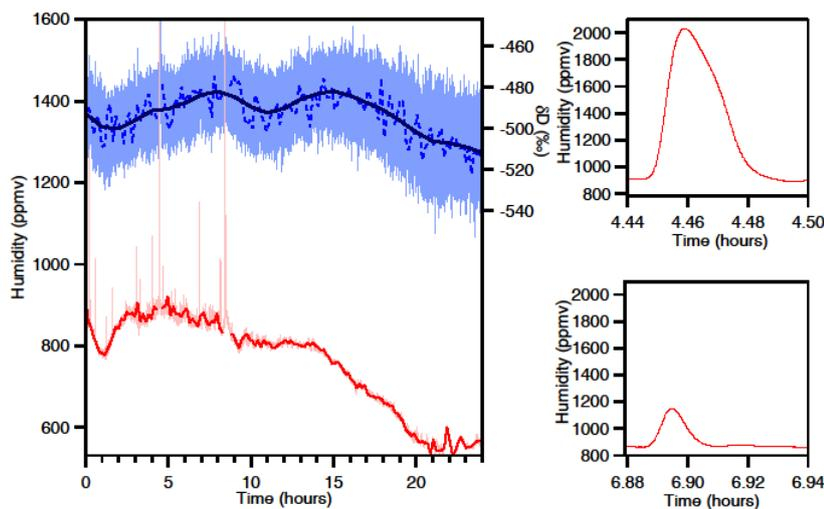
385 *Figure 5:* left : example of raw data measured by the Picarro: humidity (light red, ppmv) and  $\delta D$  (light blue, ‰), data averaged over 10 minutes for humidity (red, ppmv) and for  $\delta D$  (dashed line blue, ‰) and over 1 hour for  $\delta D$  (dark blue, ‰). Right: zoom on two “precipitation events” identified in the humidity signal of the Picarro (top, snow flake; bottom, diamond dust).
