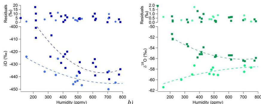
Figure 4: Measured isotopic composition for a)  $\delta D$  and b)  $\delta^{18}O$  using the PICARRO spectrometer for a fixed humidity: light circles are field calibration points, dark squares are laboratory calibration points, the dashed lines are the fit with a quadratic function and on top are the residuals compared to the fit for the entire series.
