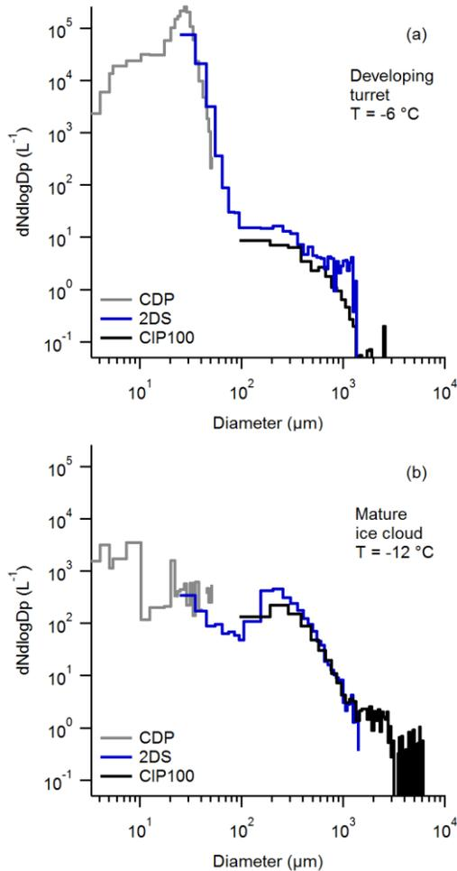
Comparison of size distributions from the CDP, 2DS and CIP100 probes during selected cloud penetrations through (a) a developing turret and (b) a mature glaciated region. The first 2 size bins from the 2DS and CIP100 were removed, as they are subject to large uncertainty, and are not used in this analysis.”
