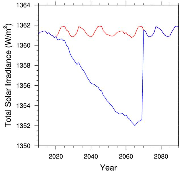
Figure1: Total solar irradiance ( $\text{W/m}^2$ ) for G3S, baseline experiment (red), solar dimming experiment (blue).
