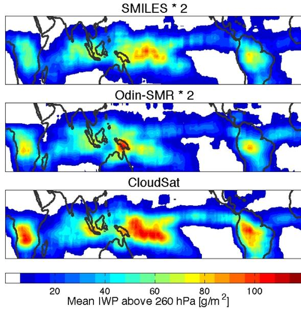
**Fig. 7.** Average pIWP<sub>260hPa</sub> for some satellite datasets. The data represent a running average over 8°/16° in latitude/longitude. SMILES and SMR means are multiplied with a factor 2.
