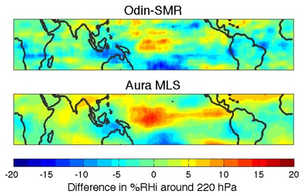
**Fig. 4.** Difference in average %RH around 220hPa between data corresponding to positive and negative MEI (positive minus negative). Data between Oct 12 and Apr 21 from complete SMR and MLS periods are included. The data represent a running average over  $6^{\circ}/12^{\circ}$  in latitude/longitude.
