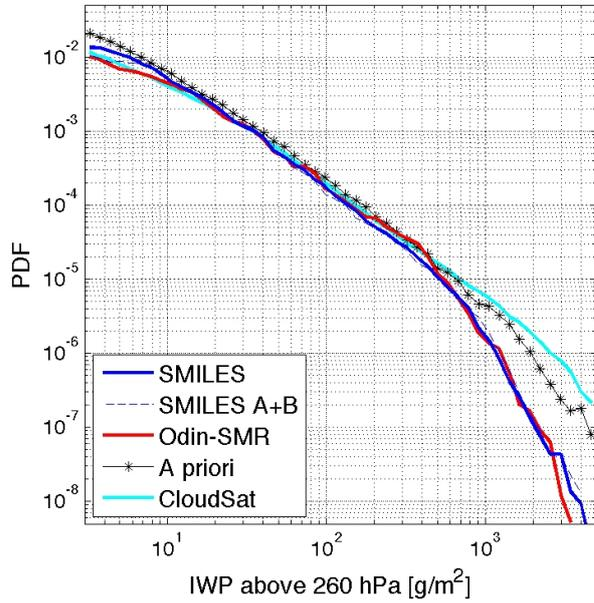
**Fig. 5.** PDFs of  $pIWP_{260hPa}$  retrievals, i.e. estimated ice column above 260 hPa. The geographical area considered is latitudes between  $30^\circ S$  and  $30^\circ N$ . The CloudSat data are averaged over 30 km to roughly match the footprint size of SMR and SMILES.
