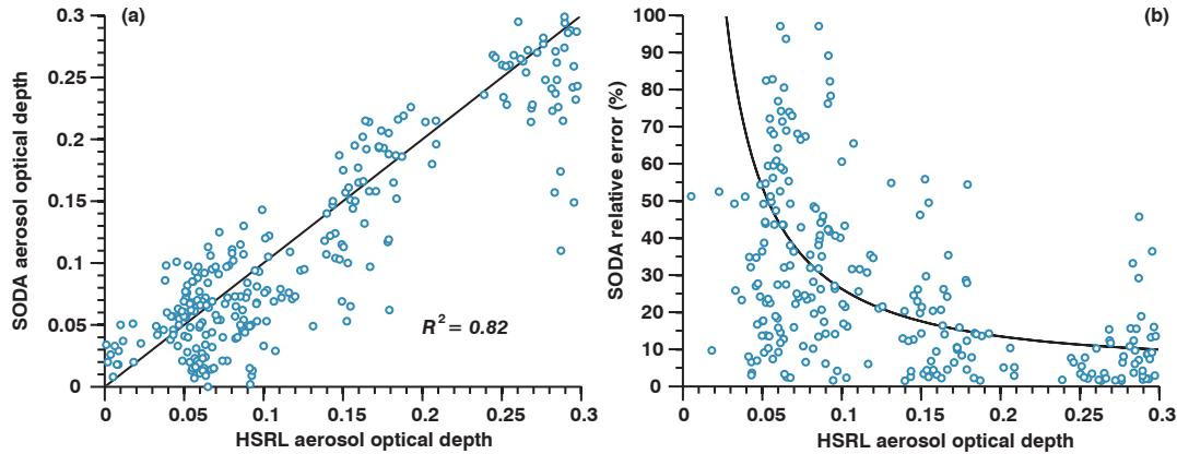
**Fig. 6** (a) A scatter plot of SODA AOD relative to AOD measured by HSRL at 532 nm. The dashed black line illustrates the 1:1 line. (b) Relative uncertainty in the SODA column lidar ratio as a function of HSRL AOD with the black line showing the least squares exponential fit as in Eq. 15 Josset et al. (2012).
