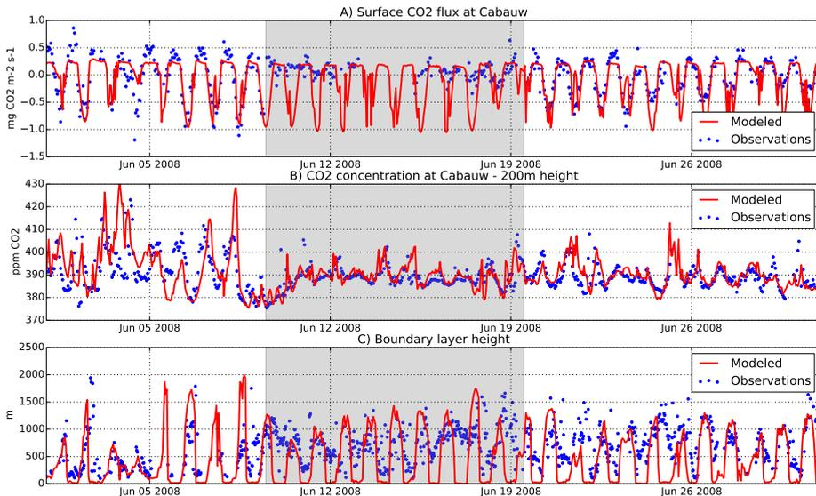
**Fig. 2.** Comparison between modeled and observed CO<sub>2</sub> fluxes, concentrations and boundary layer height for the location of Cabauw for one month in the simulated season. Performance is usually better on clear days as compared to cloudy ones, indicated in the graph with the gray background.
