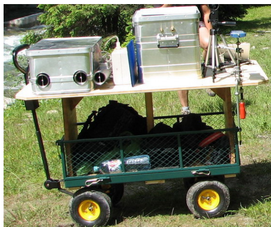
Fig. 2. Air ion detectors (left), SMPS, anemometer and GPS (middle) and field strength meter.
