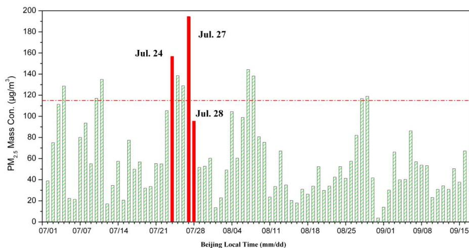
**Figure 1.** Daily variation of the  $PM_{2.5}$  concentration between Jul. and Sep/ 2008 at IAP. The dotted line represents the definition of a moderate pollution day ( $PM_{2.5}=115 \mu\text{g}/\text{m}^3$ ), and Jul. 24, 27 and 28 are highlighted.
