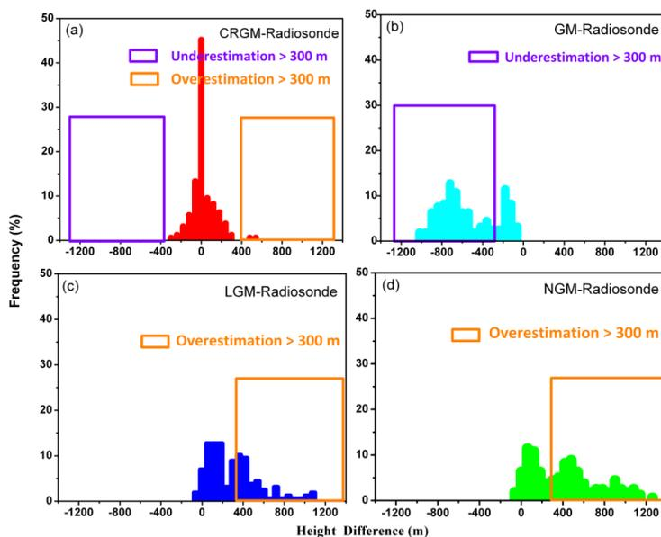
**Figure 5.** Histograms of the differences in BLH detected by radiosonde and by CRGM, NGM, LGM and GM. The X-axis is the height difference (m) between the retrieved BLH and that from radiosonde, and the Y-axis is the frequency of occurrence (%). The orange and purple regions highlight height differences of more than  $\pm 300$  m.
