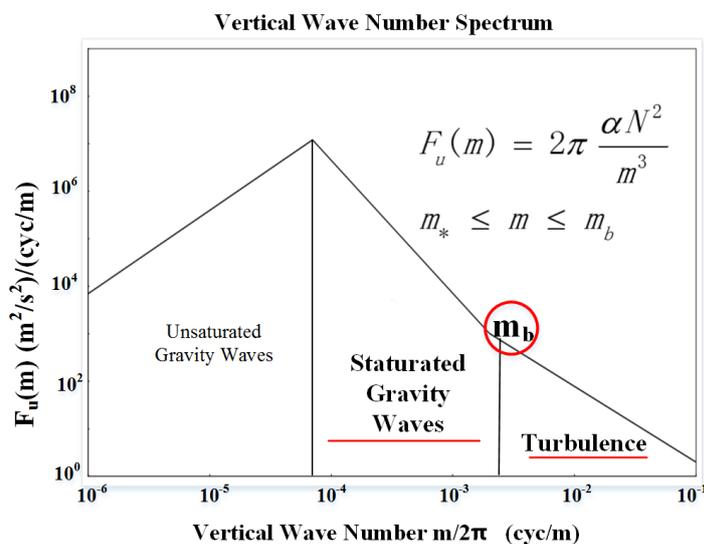
**Figure 3.** The canonical gravity wave vertical wave number spectrum of horizontal wind fluctuations. <sup>a</sup>
