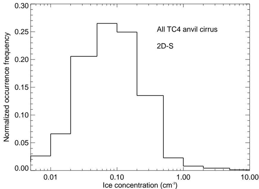
**Fig. 17.** 2D-S ice number concentration frequency distributions from all TC-4 DC-8 anvil sampling periods (over 13 h of data). The convective turrets sampled on 22 and 24 July are excluded. Ice concentrations exceeding 1–3 cm occur less than 1.4% of the time.
