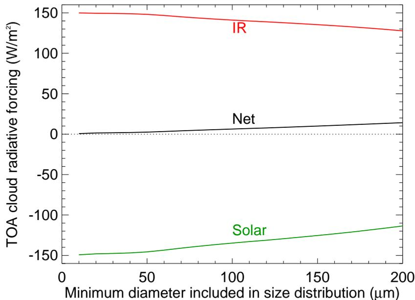
**Fig. 13.** Solar, infrared, and net top-of-atmosphere cloud radiative forcings are plotted versus the minimum size included in the ice crystal size distributions. Incrementally excluding small crystals up to a larger and larger size decreases both solar and infrared forcing, with a slight increase in net forcing. Small ( $D < 50 \mu\text{m}$ ) contribute very little to radiative forcing.
