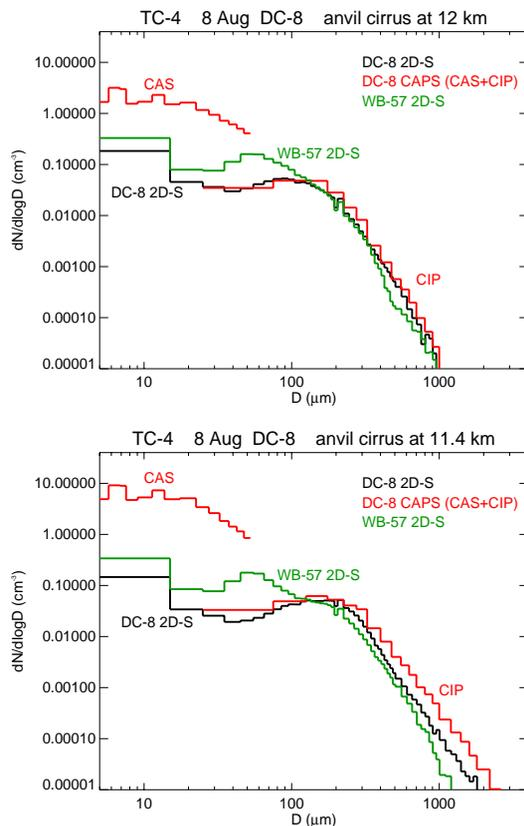
**Fig. 2.** Size distributions averaged over flight legs when WB-57 and DC-8 successively flew along the same flight legs at approximately 12 km (top) and 11.4 km (bottom) on 8 August are shown. The DC-8 CIP distribution agrees well with the 2D-S distribution; however, the concentrations of small particles indicated by CAS are 1–2 orders of magnitude higher than indicated by 2D-S.
