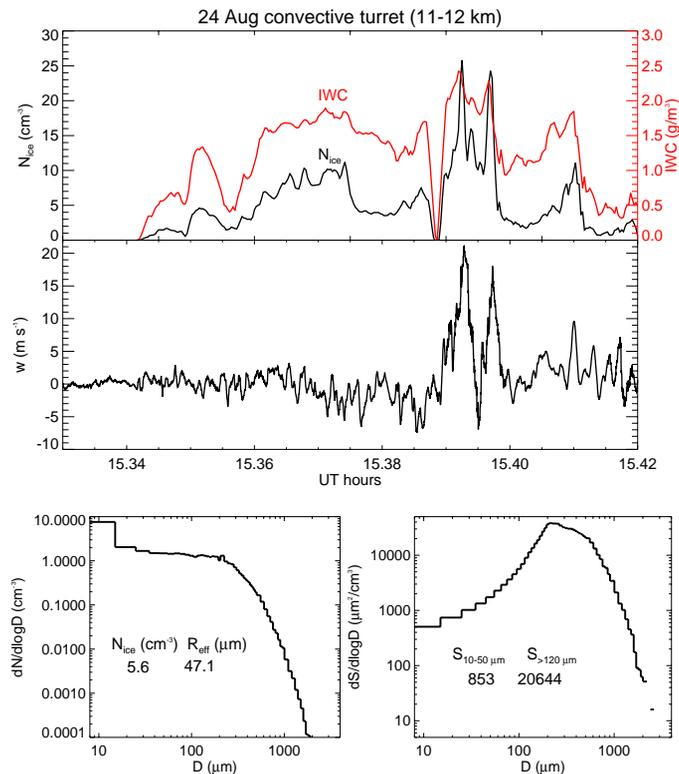
**Fig. 9.** Time series of ice concentration, and IWC (top panel) and vertical wind speed (middle panel) are shown for an active turret sampled on 24 July. Number and surface area distributions are shown in the bottom panels.
