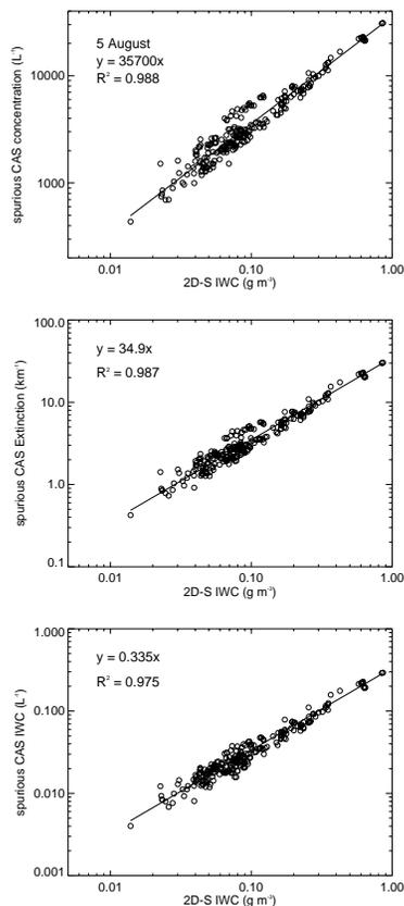
**Fig. 6.** Scatterplots of spurious CAS concentration (top), extinction (middle), and and IWC (bottom) (11–50  $\mu\text{m}$ ) versus 2D-S ice water content for time segments with relatively homogeneous clouds (see text). The lines shown are linear least-squares regression fits, and the slopes are given in the legends.
