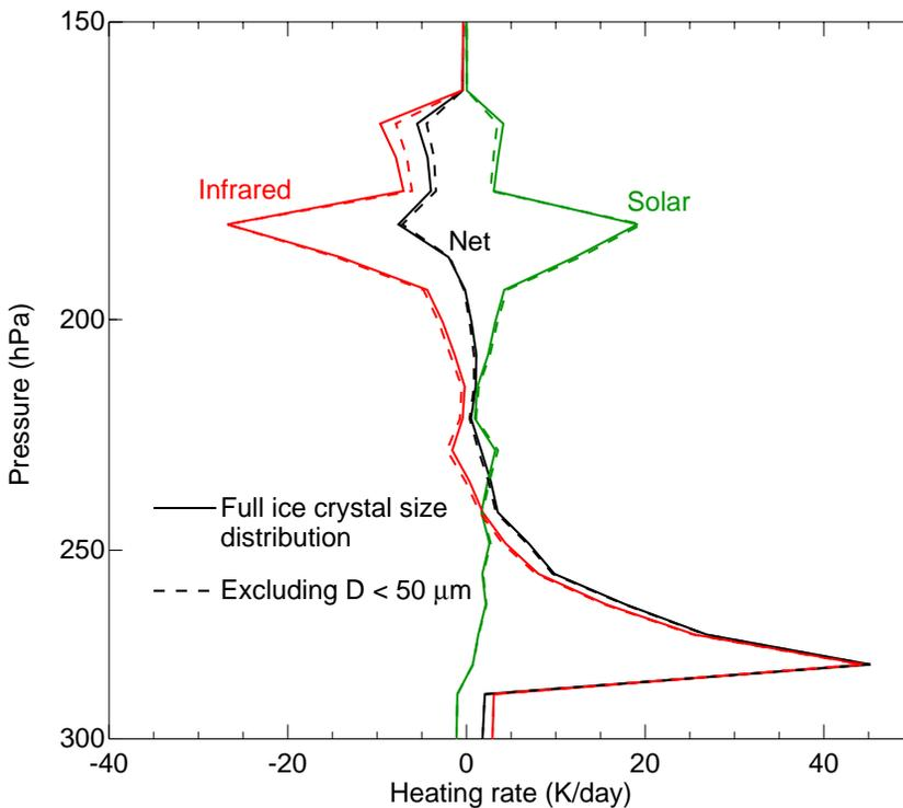
**Fig. 14.** Solar, infrared, and net cloud radiative heating rate profiles are plotted from calculations including all crystal sizes (solid) and excluding crystals smaller than  $50\ \mu\text{m}$  (dashed). The small crystals have negligible impact on radiative heating.
