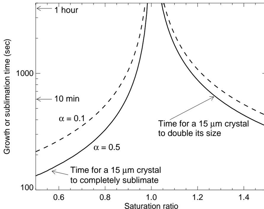
**Fig. 11.** The times required for an ice crystal to either completely sublimate (in subsaturated air) or double its size (in supersaturated air) plotted versus ice saturation ratio for two different assumed deposition coefficients. These calculations assumed a temperature of 220 K and a pressure of 200 hPa. Given the relative humidity variability typically observed in anvil cirrus, it is not surprising that the plentiful small crystals detrained from convection do not persist.
