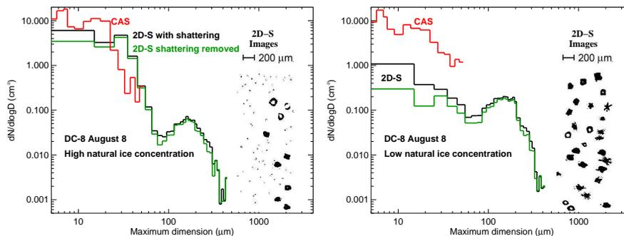
**Fig. 3.** CAPS and 2D-S size distributions (with and without shattering artifacts removed) are shown for two cases. Left panel: a case with numerous natural small crystals for which shattering has a relatively small impact on small-crystal concentration. Right panel: a case with low natural small-crystal concentrations for which shattering artifacts significantly affect the measurements.
