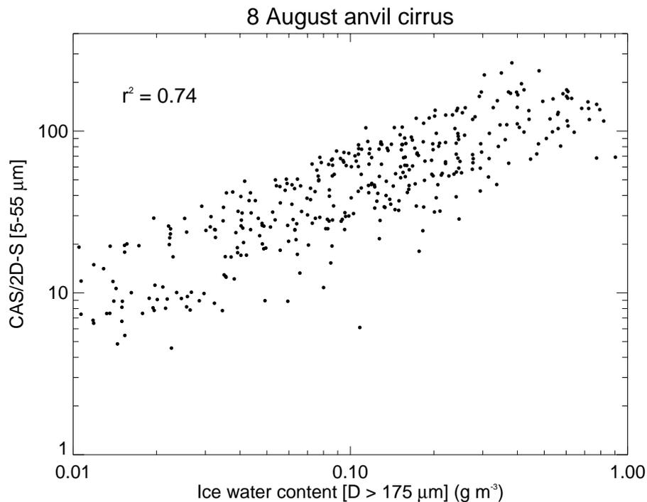
**Fig. 4.** Scatterplot of the CAS/2D-S concentration ratio versus ice water content in large ( $>175 \mu\text{m}$ ) ice crystals in the anvil cirrus sampled on 8 August. The strong correlation suggests that the CAS concentrations are exaggerated as a result of shattering artifacts.
