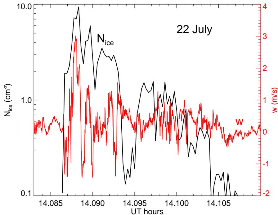
**Fig. 15.** Time series of vertical wind speed measured by MMS (red) and 2D-S ice concentration (black) in a region with high ice concentrations apparently caused by a gravity wave.
