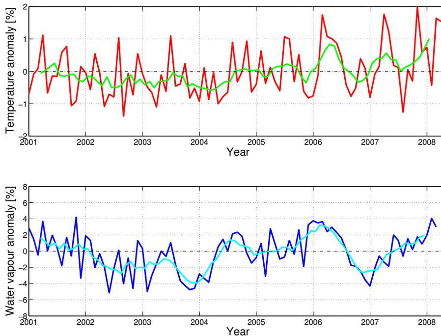
**Fig. 9.** Upper panel, ECMWF temperature anomalies measured at 100 hPa and between 20° S and 20° N (red). Overlaid is the five month running mean of the same data (green). Lower panel, the water vapour all instrument average for 30° S–30° N and 20–25 km. Overlaid is the five month running mean of the same data (cyan).
