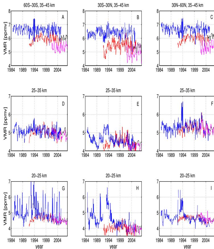
**Fig. 2.** Monthly mean water vapour time series comparison of 4 instruments in nine altitude/latitude bins; SAGE II (blue), HALOE (red), SMR (magenta), and MLS (black). The bins range from 60° S to 60° N in an altitude range from 20–45 km.
