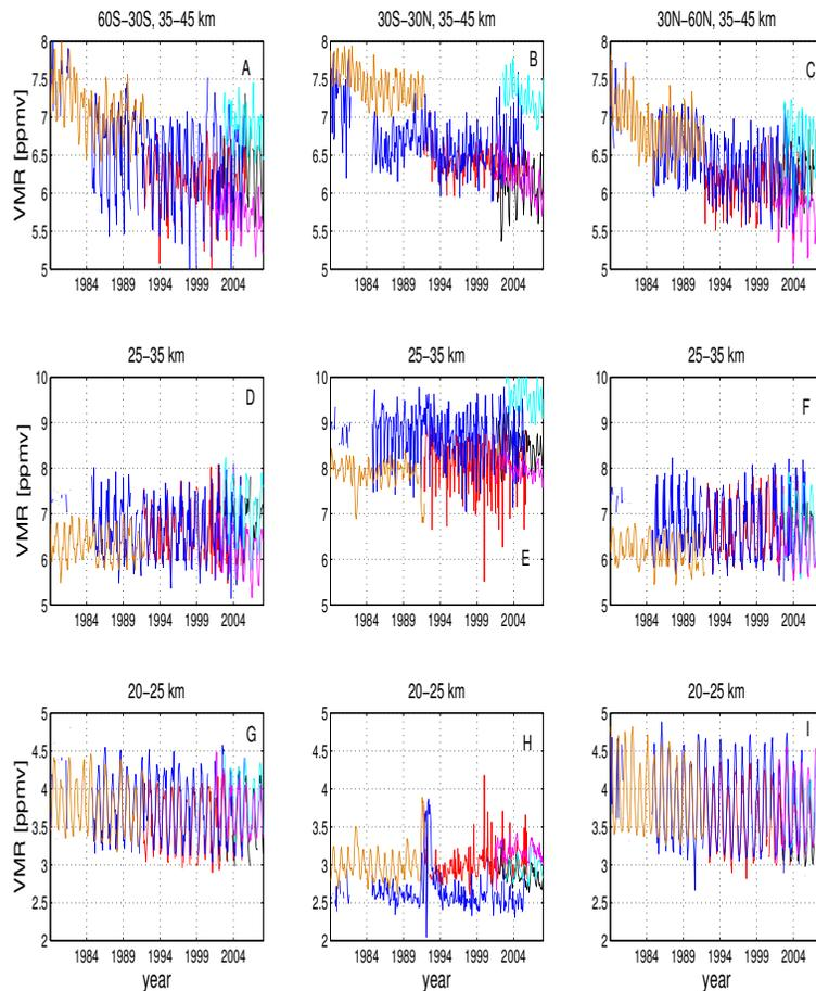
**Fig. 1.** Monthly mean ozone time series comparison of 6 instruments in nine altitude/latitude bins; SAGE I+II (blue), SBUV/2 (orange), HALOE (red), SMR (magenta), OSIRIS (black), SCIAMACHY (cyan). The bins range from 60° S to 60° N in an altitude range from 20–45 km.
