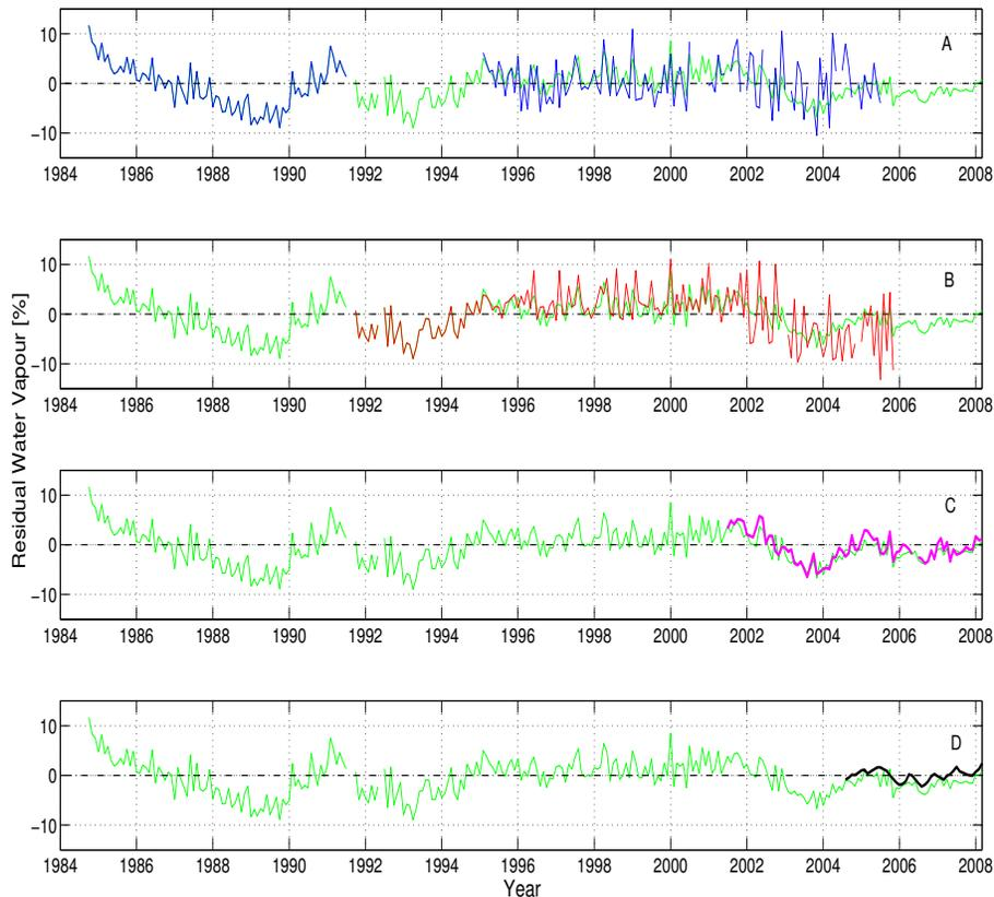
**Fig. 7.** Water vapour residuals for four instruments for the 30° S–30° N and 25–35 km bin. Shown are the SAGE I+II (blue, A), HALOE (red, B), SMR (magenta, C), MLS (black, D). Also shown under-laid is the all instrument average (green).
