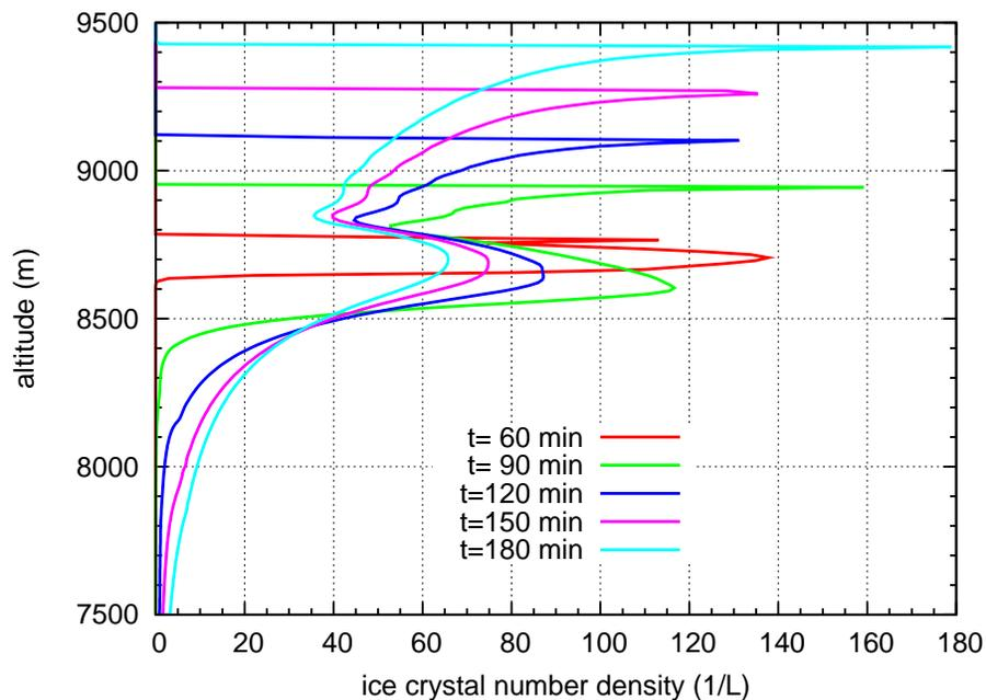
**Fig. 18.** Downward moving peak of ice crystal number density for the first nucleation event in the simulation with constant uplift of  $w=0.0\text{ m s}^{-1}$ . The peak is much more pronounced as in Fig. 17 due to higher ice crystal densities due to the stronger updraught.
