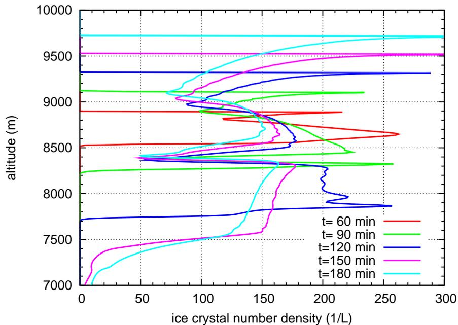
**Fig. 21.** Ice crystal number densities for  $w=0.08 \text{ m s}^{-1}$  at different simulation times. For the early simulation times, the moving peak is visible, while for  $t_s=90/120 \text{ min}$ , the in-cloud nucleation event in the vertical range  $7700 \leq z \leq 8400 \text{ m}$  appears. The ice crystals, formed in the secondary nucleation event are then dispersed over the lower part of the cloud ( $T_s=150/180 \text{ m}$ ). This leads to a layer structure of the cirrus cloud.
