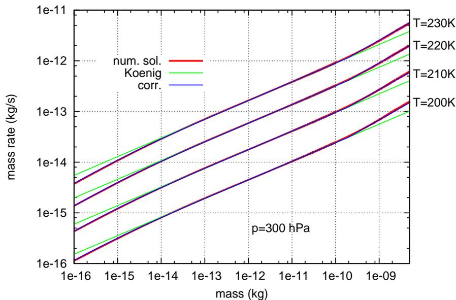
**Fig. 5.** Approximation of single ice crystal growth rates  $dm/dt$  (red) using the original Koenig ansatz (green) and the Koenig ansatz with our corrections (blue) for different temperatures ( $T=230/220/210/200\text{ K}$ ) and fixed pressure ( $p=300\text{ hPa}$ ).
