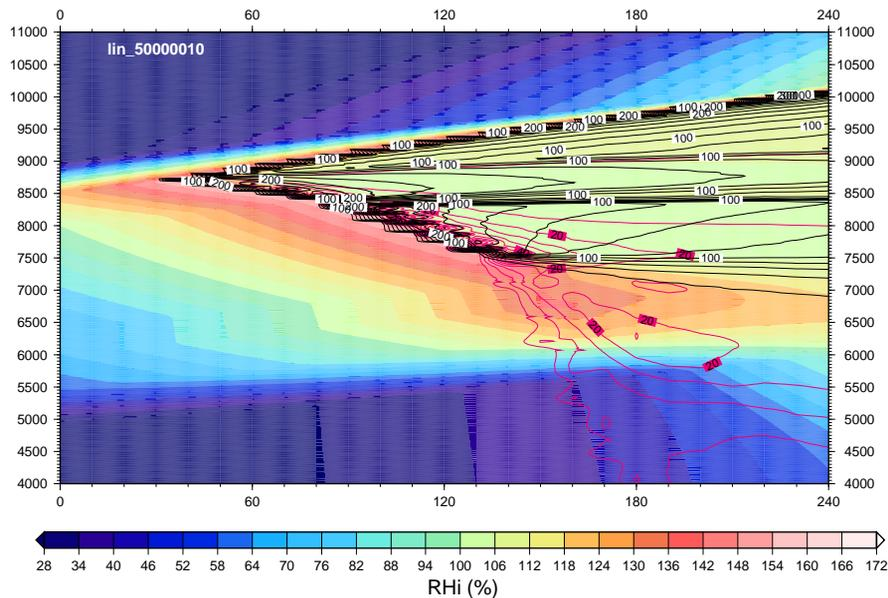
**Fig. 20.** Time evolution of the simulated cirrostratus lifted with a constant vertical velocity of  $w=0.08\text{ m s}^{-1}$ . The colours indicate relative humidity wrt ice, while lines indicate ice crystal number densities (black, in  $\text{L}^{-1}$ ) and ice water content (purple, in  $\text{mg m}^{-3}$ ).
