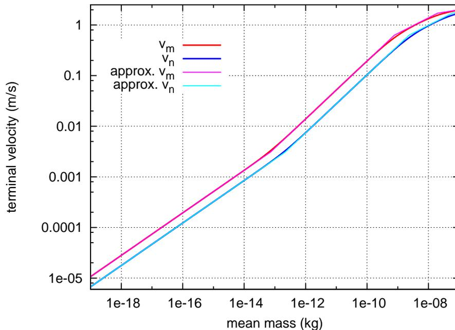
**Fig. 6.** Mean terminal velocities  $v_m$ ,  $v_n$  for  $r_0=3$  and the approximations by using the expressions of general moments as in Eq. (50) as piecewise functions.
