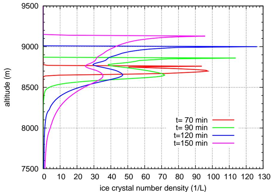
**Fig. 17.** Downward moving peak of high ice crystal number densities formed by the first homogeneous nucleation event at  $t \approx 60$  min in the reference simulation (i.e. constant uplift of  $w = 0.05 \text{ m s}^{-1}$ ). At the top of the cloud there is continuous nucleation, indicated by the high peak values of ice crystal number density.
