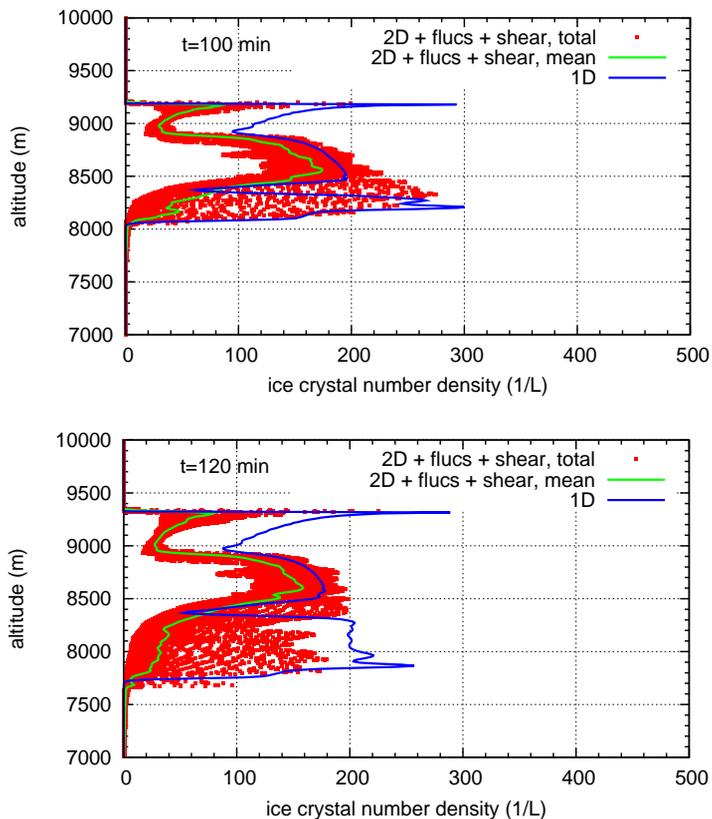
**Fig. 26.** Ice crystal number densities for a vertical updraught of  $w=0.08 \text{ m s}^{-1}$  with fluctuations and wind shear (red dots: all grid points, green line: mean value) and in the corresponding 1-D simulation (blue line) for  $t=100$  min (top) and 120 min (bottom), respectively. In contrast to the simulations including only temperature fluctuations (Fig. 24), here the incloud nucleation events at the cloud bottom occur; however, they are weaker than in the pure 1-D simulations.
