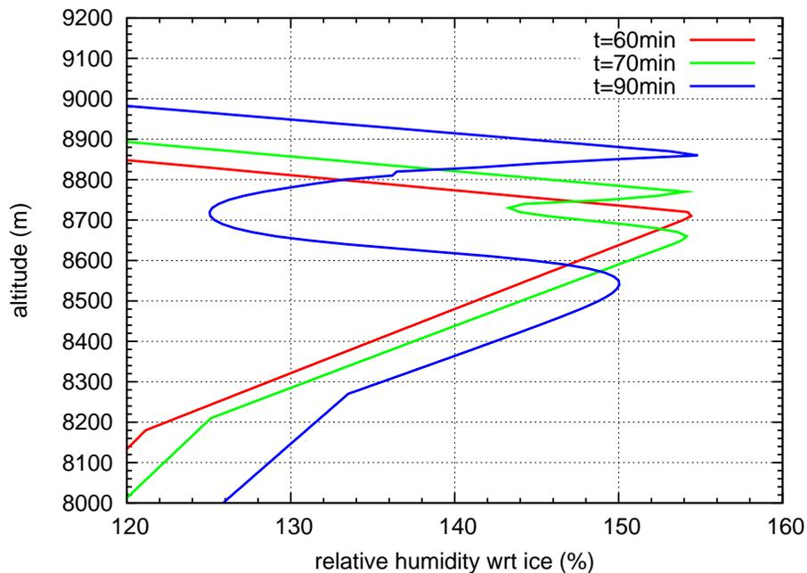
**Fig. 16.** Temporal evolution of the vertical RHi profiles for simulation time  $60 \leq t \leq 90$  min. The notch of the profile due to ice crystal growth is represented clearly, while the supersaturation at the cloud top remains.
