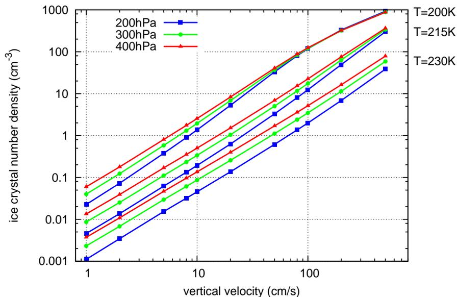
**Fig. 10.** Box model calculations for the homogeneously formed ice crystal number densities depending on the vertical velocity and on the temperature. For the simulations, we assume a fixed width for the aerosol size distribution of  $\sigma_r=1.4$  and a geometric mean radius of  $r_m=25$  nm. Here, the impact of pressure on the formation of ice crystals is shown using values of  $p=200/300/400$  hPa.
