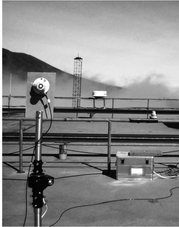
Fig. 1. The measuring system, movable vertically placed and horizontally fixed Kipp & Zonen dual band biometer, at site of ALOMAR Observatory.
