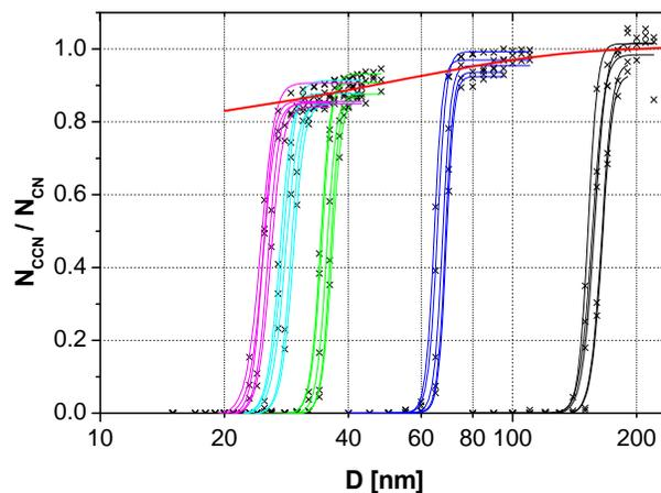
**Fig. 1.** CCN efficiency spectra obtained from 5 calibration experiments with ammonium sulfate aerosol performed during the campaign (data points and CDF fits). The red line is the asymptotic function that was used to correct for different counting efficiencies of the CPC and the CCNC ( $f_{\text{corr}}$ ).
