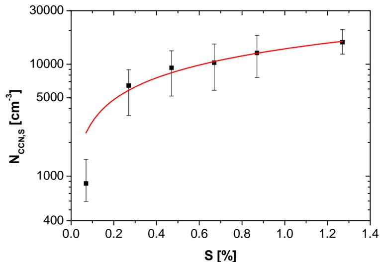
**Fig. 10.** CCN number concentrations ( $N_{\text{CCN},S}$ ) averaged over the entire campaign and plotted against water vapor supersaturation ( $S$ ). The data points are median values, and error bars extend to lower and upper quartiles. The red line is a classical power law fit of the function  $N_{\text{CCN},S} = N_{\text{CCN},1} \cdot (S/(1\%))^k$  with the best fit parameters  $N_{\text{CCN},1} = 13\,699 \text{ cm}^{-3}$  and  $k = 0.65$  ( $R^2 = 0.97$ ,  $n = 6$ ).
