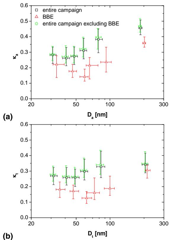
**Fig. 7.** Hygroscopicity parameters **(a)** for the CCN-active particles ( $\kappa_a$ ) and **(b)** for the total aerosol ( $\kappa_t$ ) averaged over different periods: the entire campaign, the biomass burning event and the campaign excluding the biomass burning event. The data points are median values corresponding to a given level of supersaturation, and the error bars extend to lower and upper quartiles.
