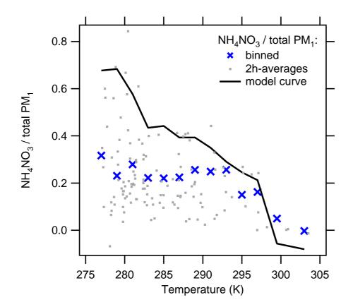
**Fig. 5.** Measured ratio of  $NH_4NO_3$  mass concentration to total aerosol mass concentration as a function of temperature, binned into temperature intervals. The dots indicate the two hour averages. The solid represents a model curve with total available nitrate and ammonia as fit parameters (for details see text).
