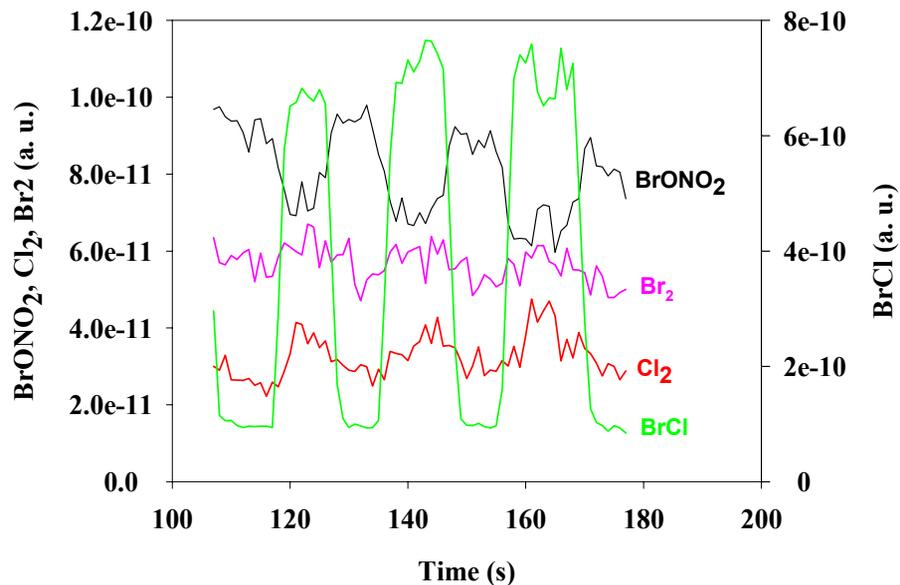
**Fig. 6.** BrONO<sub>2</sub> and products profiles in gas phase versus time ( $T = 6.4^{\circ}\text{C}$ ,  $(\text{NaCl}) = 0.1 \text{ M}$ ).
