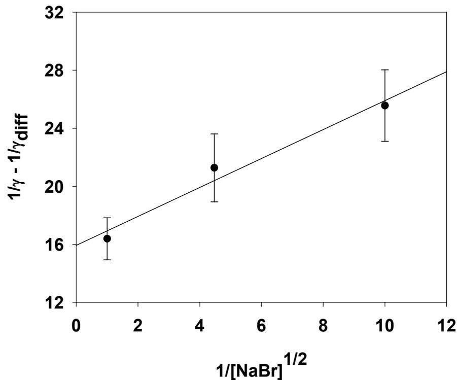
**Fig. 7.** Plot of uptake coefficients for BrONO<sub>2</sub> according to Eq. (13). The intercept is the inverse of the mass accommodation coefficient  $\alpha$ .  $T=273\pm 1$  K. The error bars are given at the  $1\sigma$  level.
