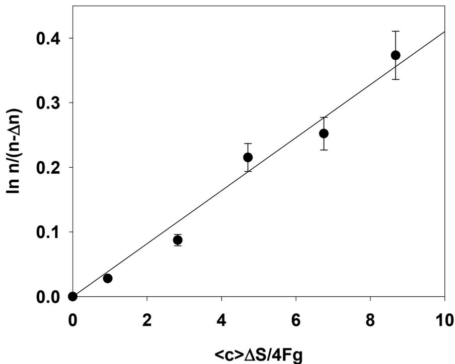
**Fig. 1.** Typical plots of  $\ln(n/n - \Delta n)$  versus  $\langle c \rangle \Delta S / 4F_g$  for ClONO<sub>2</sub> on a 0.05 M NaBr solution at 277 K. The slope is  $\gamma$  according to Eq. (5).
