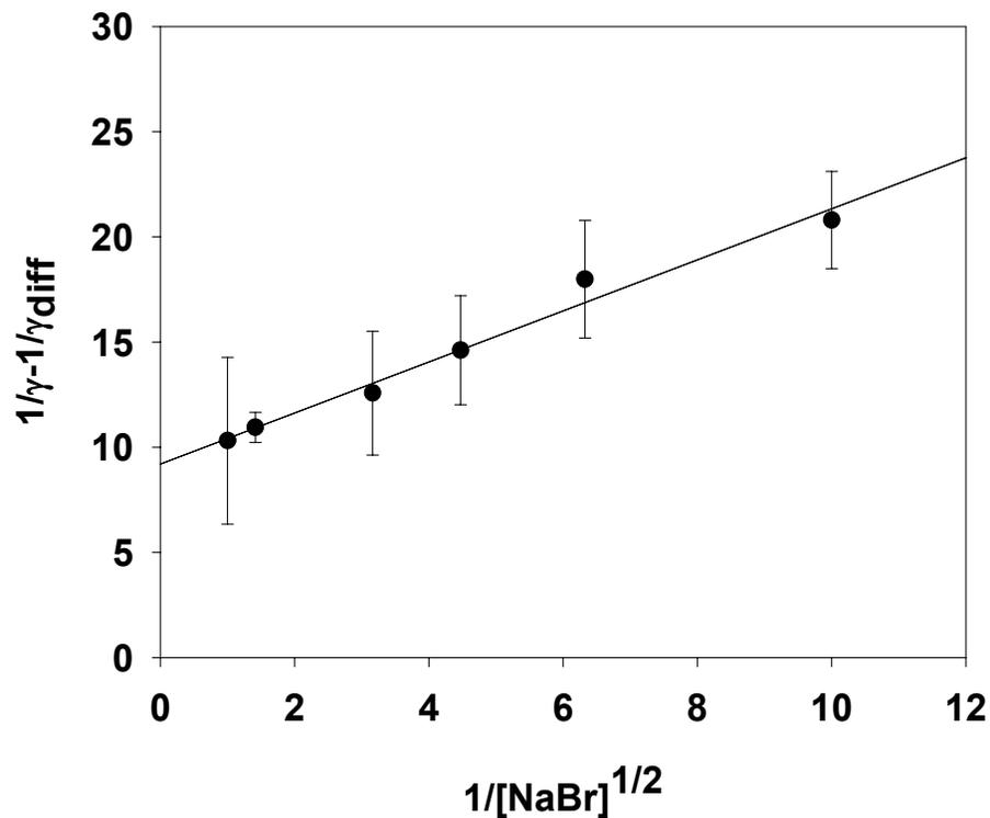
**Fig. 3.** Plot of uptake coefficients for ClONO<sub>2</sub> according to Eq. (13). The intercept is the inverse of the mass accommodation coefficient  $\alpha$ .  $T=274.5\pm 1$  K. The error bars are given at the  $1\sigma$  level.
