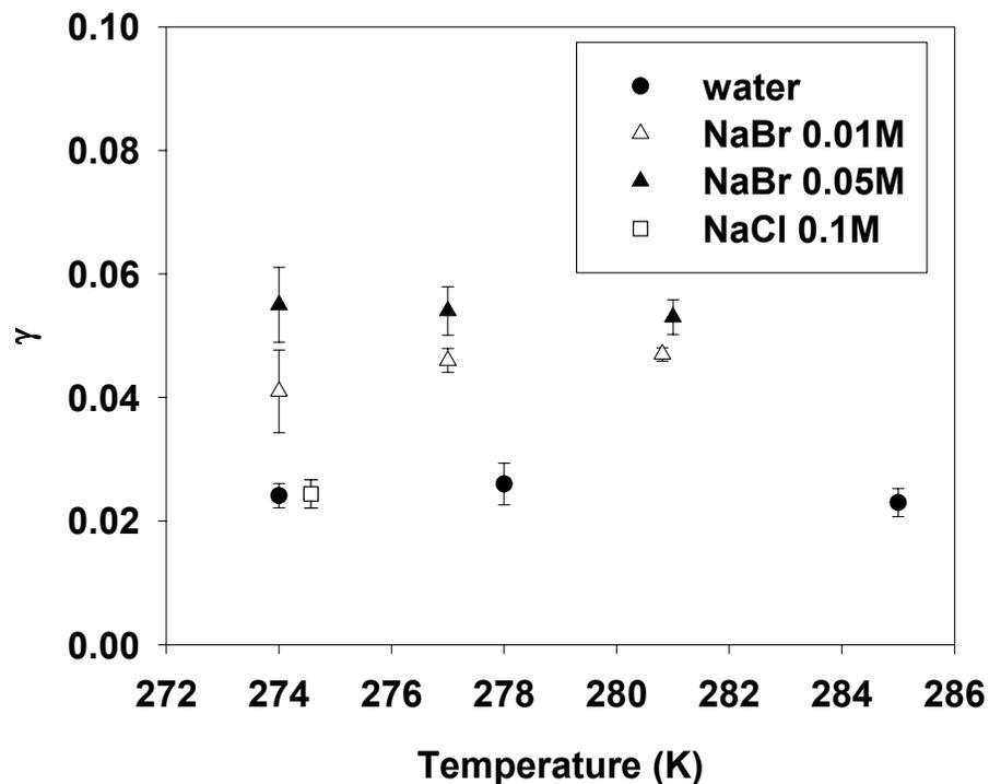
**Fig. 2.** ClONO<sub>2</sub> uptake coefficient as a function of temperature. The error bars are given at 1 $\sigma$  level. (black dot: water; triange: NaBr 0.01M ; black triangle: NaBr 0.05M; square: NaCl 0.1M).
