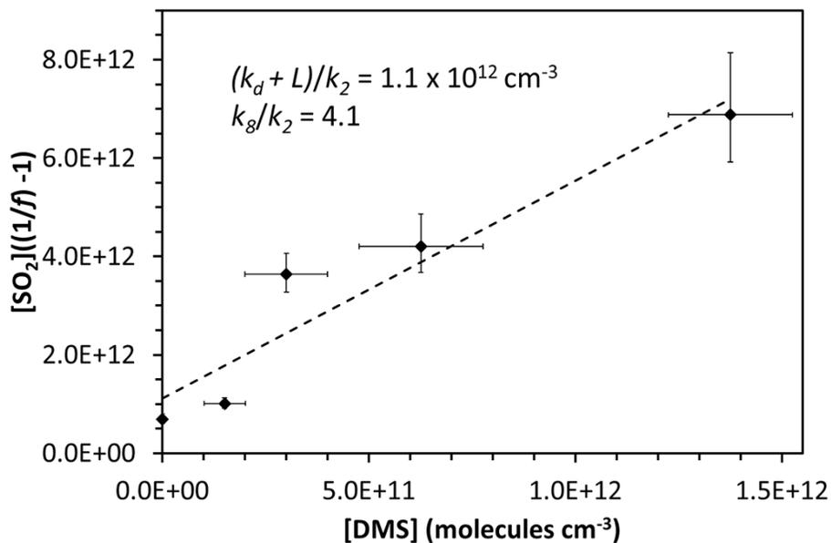
**Figure 6.** Application of Eq. (4) to derive rate constants for reaction of ISOP-SCI with DMS ( $k_8$ ) relative to that for reaction with  $\text{SO}_2$ .
