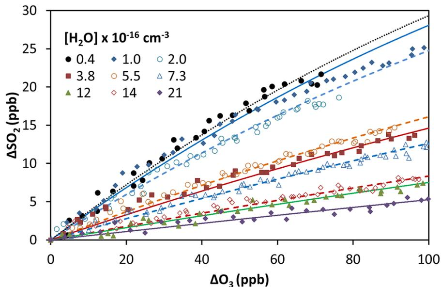
**Figure 2.** Cumulative consumption of  $\text{SO}_2$  and  $\text{O}_3$ ,  $\Delta\text{SO}_2$  vs.  $\Delta\text{O}_3$ , for the ozonolysis of isoprene in the presence of  $\text{SO}_2$  at a range of water vapour concentrations, from  $4 \times 10^{15} \text{ cm}^{-3}$  to  $2.1 \times 10^{17} \text{ cm}^{-3}$ . Symbols are experimental data corrected for chamber dilution. Lines are smoothed fits to the experimental data.
