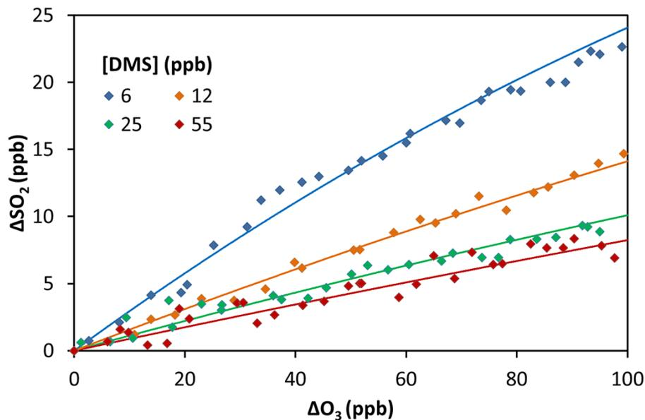
**Figure 5.** Cumulative consumption of  $SO_2$  and  $O_3$ ,  $\Delta SO_2$  vs.  $\Delta O_3$ , for the ozonolysis of isoprene in the presence of  $SO_2$  at a range of DMS concentrations, from 6 to 55 ppbv.  $[H_2O]$  in all experiments was  $< 9 \times 10^{15} \text{ cm}^{-3}$ . Markers are experimental data, corrected for chamber dilution. Solid lines are smoothed fits to the experimental data.
