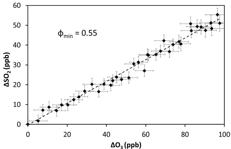
**Figure 1.**  $\Delta\text{SO}_2$  vs.  $\Delta\text{O}_3$  during the excess  $\text{SO}_2$  experiments ( $[\text{H}_2\text{O}] < 5 \times 10^{15} \text{ cm}^{-3}$ ). The gradient determines the minimum SCI yield ( $\phi_{\min}$ ) from isoprene ozonolysis.
