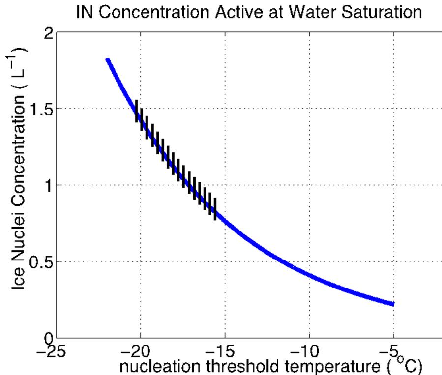
**Figure 2.** IN number concentration active at water saturation vs. temperature based on the empirical relationship derived in DeMott et al. (2010) (blue line). Black vertical lines indicate threshold temperatures for nucleation in the 16 IN bins. IN increments between lines indicate the additional IN available for nucleation at colder temperatures.
