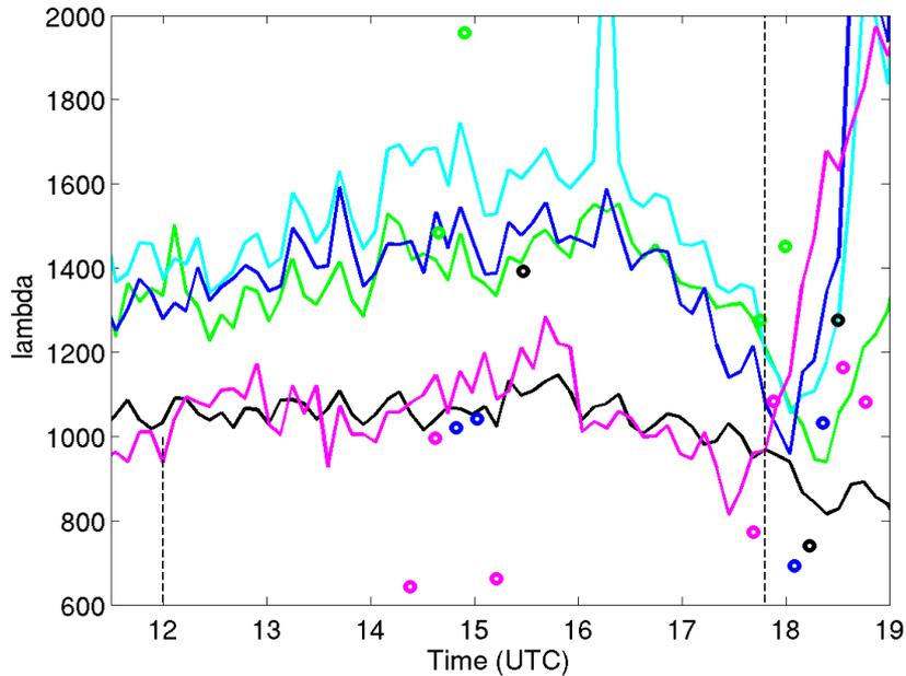
Figure 3: Temporal evolution of  $\Lambda$  observed (open circles) and obtained by LES (continuous lines) at different heights (same color code than for other figures).
