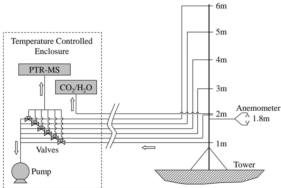
**Fig. 1.** Schematic of tower and sampling arrangement. All PTR-MS lines are equidistant (12 m) from inlet to instrument.
