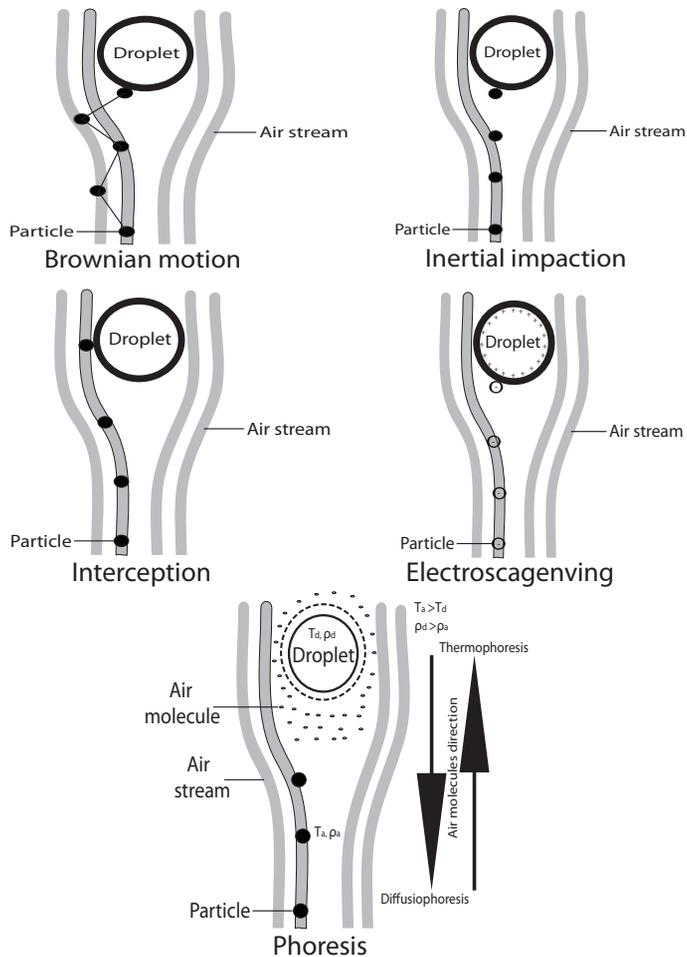
**Fig. 1.** Diagram of the different collisions pathways between aerosol particles and cloud droplets relevant to contact freezing (Ladino, 2011).
