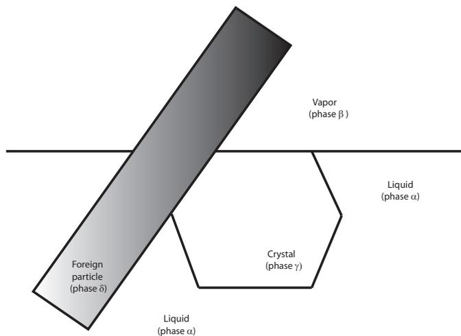
**Fig. 4.** Mechanism of contact freezing based on the different phases interactions (Djikaev and Ruckenstein, 2008).
