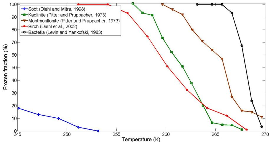
**Fig. 7.** Comparison of different contact freezing experiments conducted in a wind tunnel. The blue color represent the experiments done with soot particles, green with kaolinite, brown with montmorillonite, red with pollen and black with bacteria (Pitter and Pruppacher, 1973; Levin and Yankofsky, 1983; Diehl and Mitra, 1998; Diehl et al., 2002).
