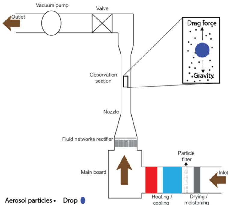
**Fig. 6.** Schematic of the wind tunnel experimental setup and its major components (Vohl et al., 1999).
