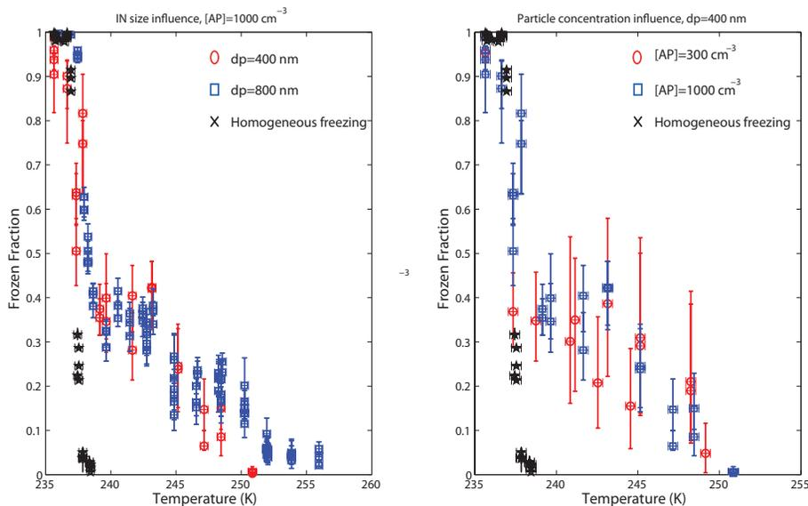
**Fig. 11.** Experimental frozen fraction on contact freezing as a function of temperature conducted in CLINCH. The cloud droplets have a residence time of 5 s. The left panel shows the comparison of two different particle sizes and the right panel the comparison of two different aerosol particle concentrations. The black stars represent the homogeneous freezing data.  $dp$  refers to the aerosol particle diameter and  $[AP]$  to the aerosol particle concentration.
