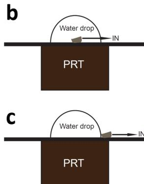
**Fig. 5.** (a) Schematic with the cold plate experimental setup (left). (b) Location of the IN for an immersion freezing (top right) and (c) for a contact freezing experiment (bottom right) (Shaw et al., 2005).
