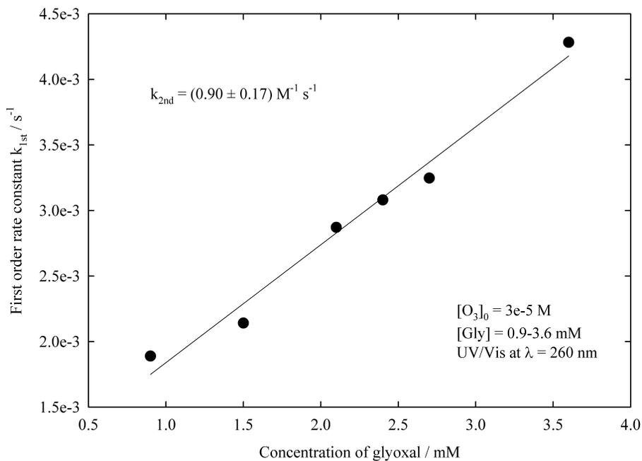
**Fig. 3.** Pseudo-first order rate constants  $k_{1st}$  plotted over the concentration of glyoxal during the reaction with ozone. The slope corresponds to  $k_{2nd} = (0.90 \pm 0.17) M^{-1} s^{-1}$ .
