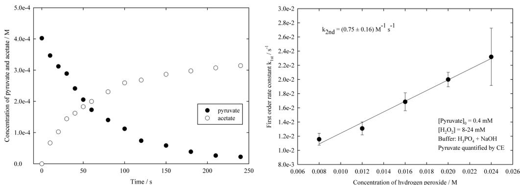
**Fig. 5.** Left: concentration-time profiles of pyruvate and acetate during the reaction with H<sub>2</sub>O<sub>2</sub> at pH 7 for  $c(\text{pyruvate}) = 0.4 \text{ mM}$  and  $c(\text{H}_2\text{O}_2) = 12 \text{ mM}$ . Right: pseudo-first order constants  $k_{1st}$  plotted over the concentration of hydrogen peroxide for the reaction with pyruvate at pH 7.
