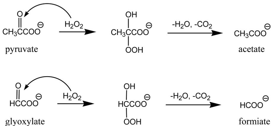
**Scheme 3.** Reaction mechanism of pyruvate and glyoxylate + H<sub>2</sub>O<sub>2</sub>.
