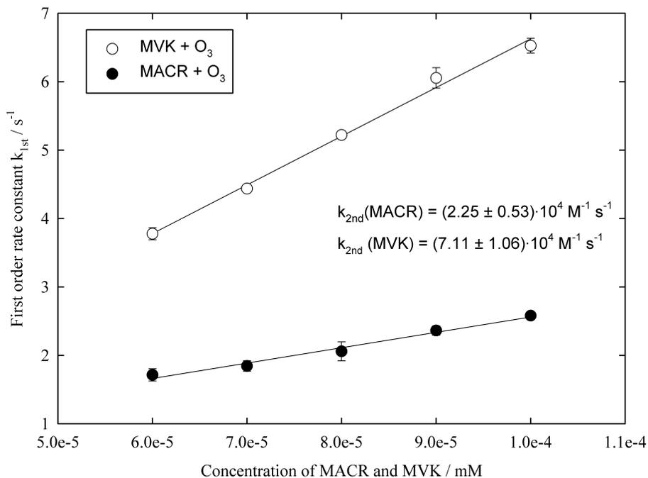
**Fig. 4.** Pseudo-first order rate constants  $k_{1st}$  plotted over the concentration of methacrolein and methyl vinyl ketone for the reaction with ozone.
