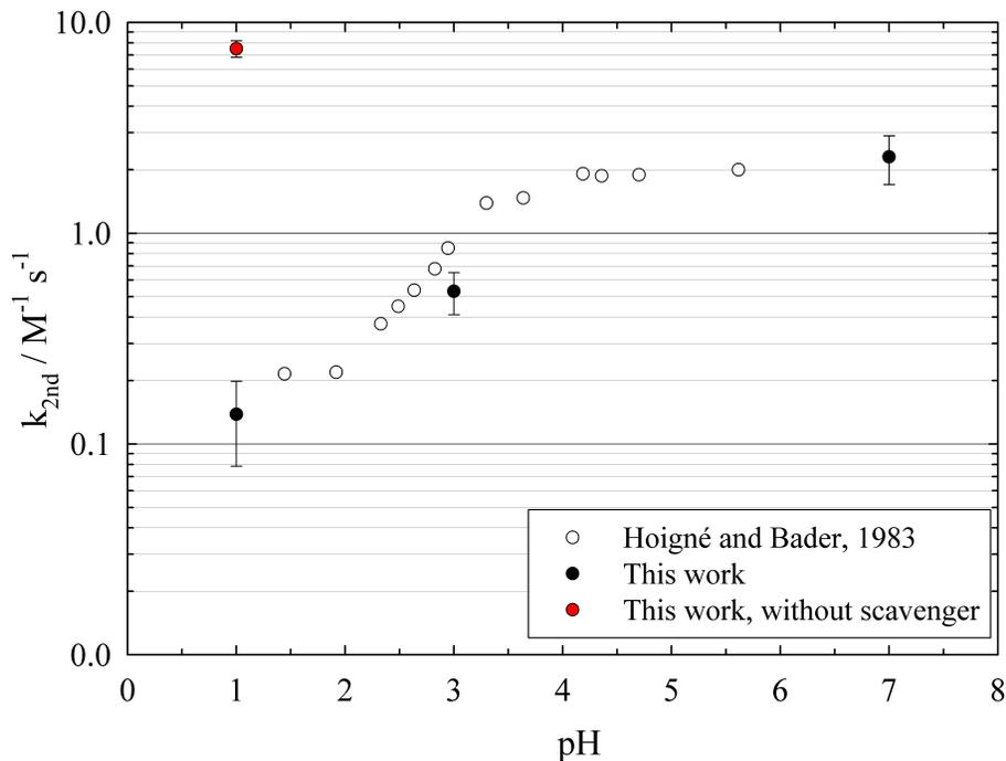
**Fig. 2.** Rate constants ( $M^{-1} s^{-1}$ ) plotted as a function of pH value for the reaction of glyoxylic acid/glyoxylate with ozone. Hoigné and Bader (1983b, white dots); this work (black dots); no scavenger used in this work (red dot).
