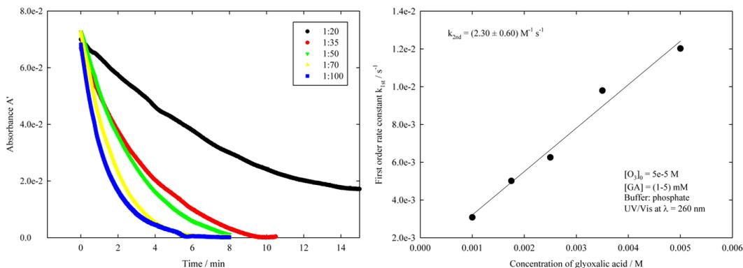
**Fig. 1.** Left: absorbance-time profiles of ozone during the reaction with glyoxylate at pH 7. The initial concentration of ozone was about  $c(\text{O}_3) = 5 \times 10^{-5} \text{ M}$ . Right: pseudo-first order rate constants  $k_{1\text{st}}$  plotted over the concentration of glyoxylate.
