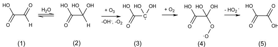
**Scheme 1.** Proposed oxidation mechanism of (hydrated) glyoxylic acid exposed to ozone in an aqueous environment.
