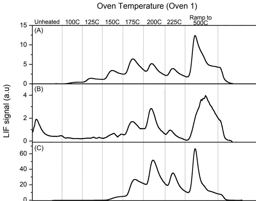
**Fig. 7. (A):** Calibration profile obtained from average of six PTD profiles using Oven 1 program for denuder loaded with pure  $\text{HgCl}_2$ . **(B):** Dissociation profiles obtained using Oven 1 program for “close in” airship sample collected 28 February 2008. **(C)** Dissociation profiles obtained using Oven 1 program for stack sample collected 29 February 2008.
