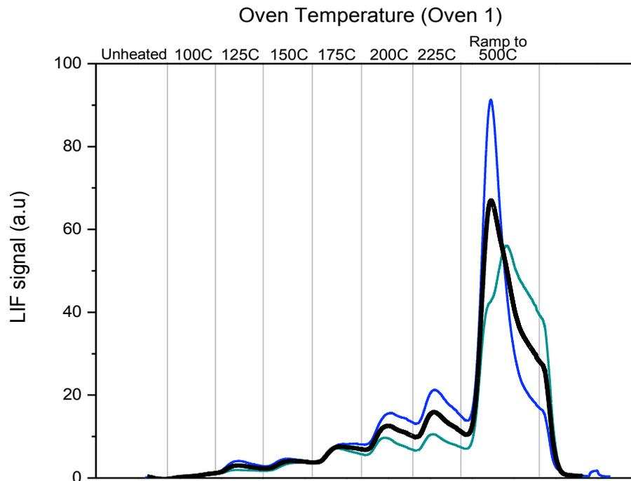
**Fig. 2.** Two PTD profiles using Oven 1 program for an uncoated tubular denuder loaded with pure  $\text{HgCl}_2$ . Denuders were loaded by flowing  $\text{N}_2$  over pure  $\text{HgCl}_2$  for 1 min at 520 sccm. The average of the two profiles is also shown.
