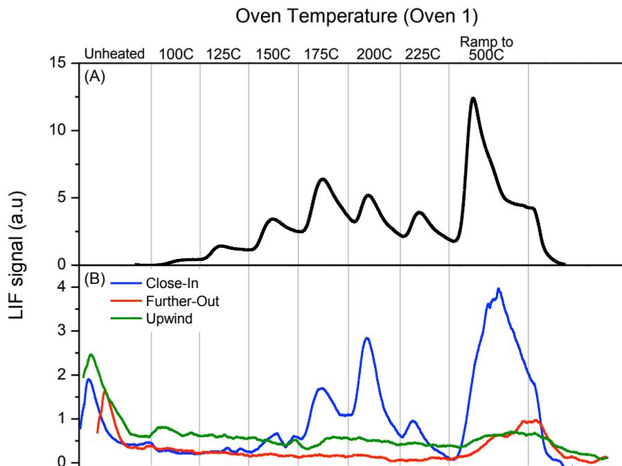
**Fig. 6. (A):** Calibration profile obtained from average of six PTD profiles using Oven 1 program for denuder loaded with pure  $\text{HgCl}_2$ . **(B):** Dissociation profiles obtained using Oven 1 program for airship samples collected 28 February 2008.
