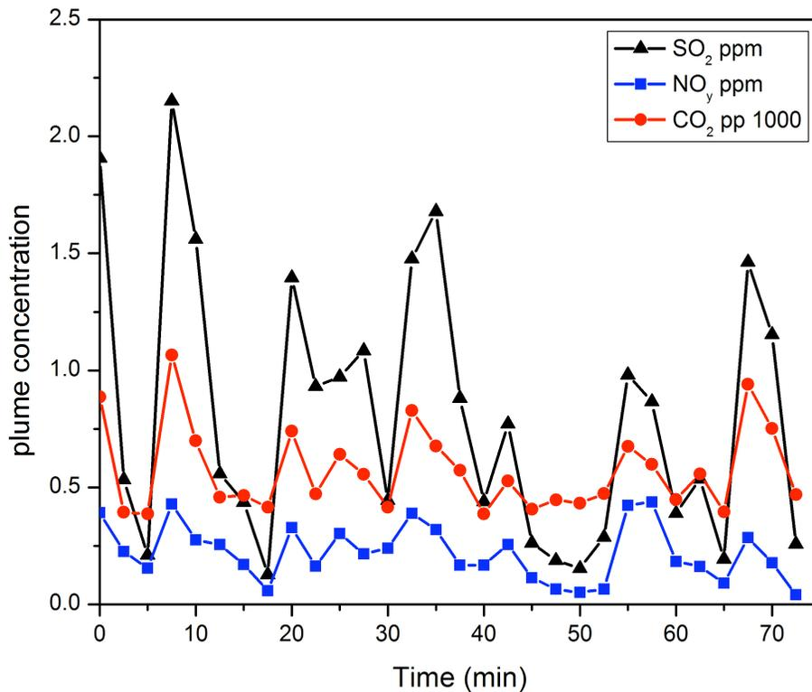
**Fig. 8.** “Background corrected” Concentrations of SO<sub>2</sub>, NO<sub>y</sub> and CO<sub>2</sub> as measured by the airship’s sampling system during the “close in” sampling run on 28 February.
