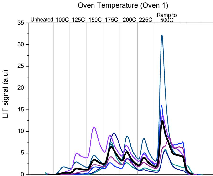
**Fig. 1.** Six PTD profiles using Oven 1 program for an uncoated tubular denuder loaded with pure  $\text{HgCl}_2$ . Denuders were loaded by flowing  $\text{N}_2$  over pure  $\text{HgCl}_2$  for 1 min at 135 sccm. The average of the six profiles is also shown.
