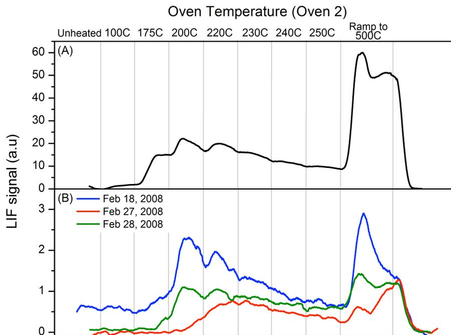
**Fig. 4.** (A): Calibration profile obtained using Oven 2 program for denuder loaded with pure  $\text{HgCl}_2$ . (B): Dissociation profiles obtained using Oven 2 program for stack samples collected 18, 27, and 28 February 2008.
