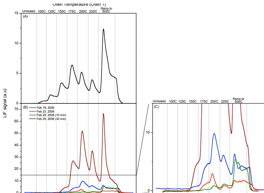
**Fig. 5.** (A): Calibration profile obtained from average of six PTD profiles using Oven 1 program for denuder loaded with pure HgCl<sub>2</sub>. (B) and (C): Dissociation profiles obtained using Oven 1 program for stack samples collected 18, 23, and 29 February 2008.
