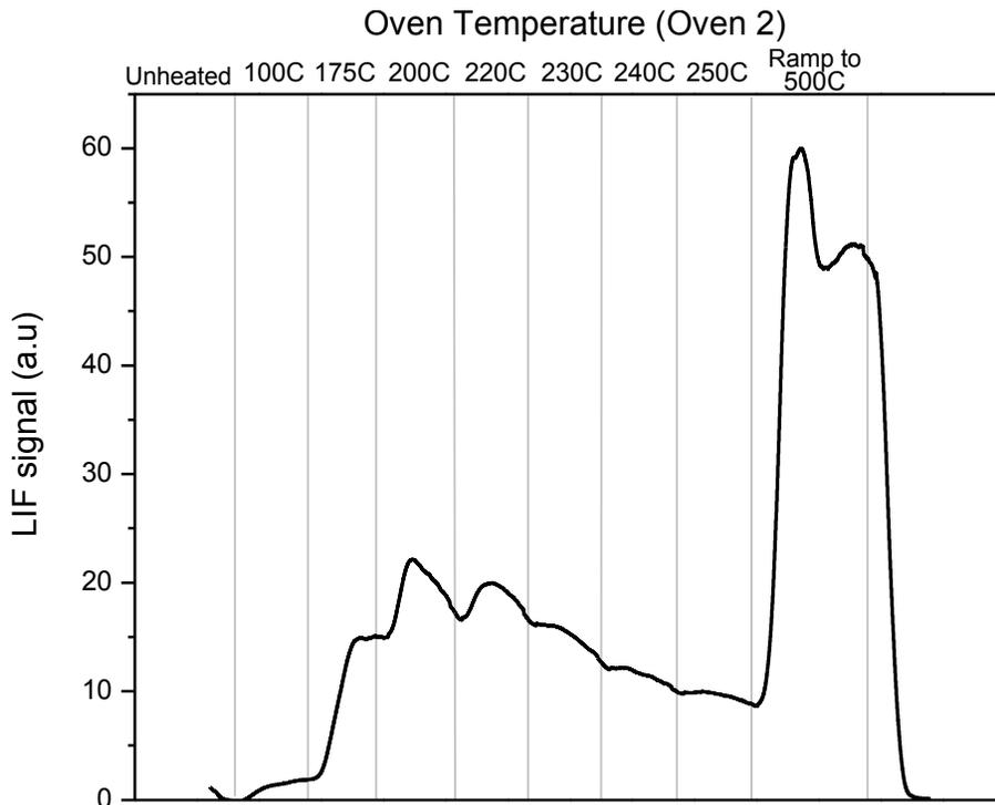
**Fig. 3.** PTD profiles using Oven 2 program for an uncoated tubular denuder loaded with pure  $\text{HgCl}_2$ . The denuder was loaded by flowing  $\text{N}_2$  over pure  $\text{HgCl}_2$  for 1 min at 520 sccm.
