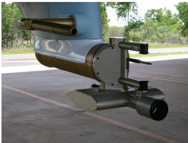
Fig. 3. Port pylon of the Egrett. In the foreground is the CAPS probe; above and to the left (as viewed), is the aerosol inlet.
