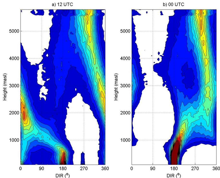
**Fig. 3.** Mean frequency distribution of wind directions at Antofagasta (Cerro Moreno Airport) at **(a)** 12:00 UTC (08:00 LT) and **(b)** 00:00 UTC (20:00 LT) as a function of standard height. A total of 5707 days in the 1961–1987 period was considered in the analysis for which 2-daily upper-air observations were available.
