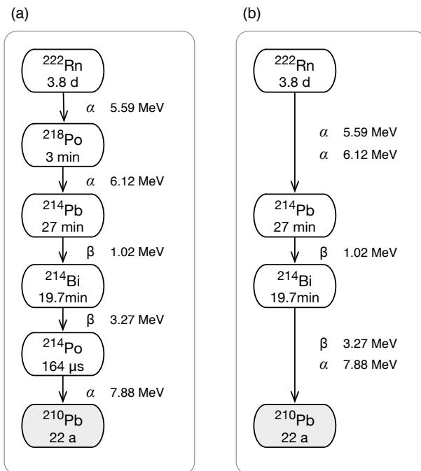
**Fig. 2.** **(a)** Radioactive decay of radon and its progeny. The half-life, decay type and decay energy of each species are also listed. **(b)** The simplified decay chain considered in our simulations.
