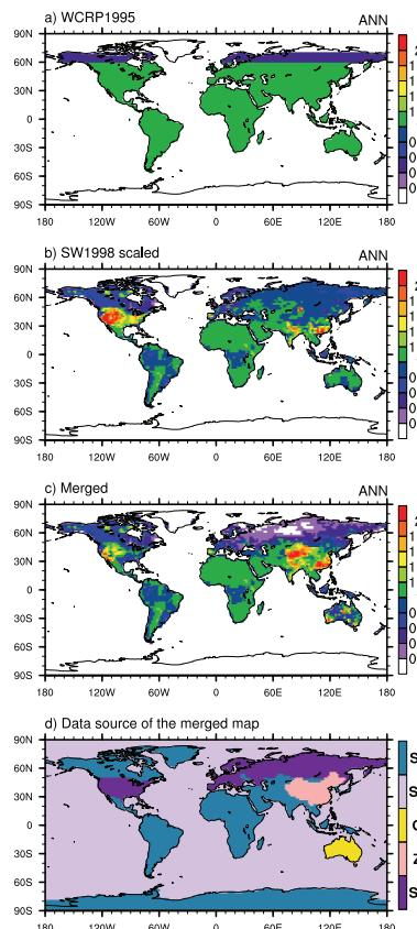
**Fig. 1. (a–c)** Radon emission setups considered in this study. The quantity shown is the annual mean atom number flux (unit:  $\text{atom cm}^{-2} \text{s}^{-1}$ ). **(d)** Data source of the merged emission map shown in **(c)**. S1 stands for Schery and Wasiolek (1998) (scaled), S2 for Schery and Huang (2004), G for Griffiths et al. (2010), Z for Zhuo et al. (2008), and S3 for Szegvary et al. (2007).
