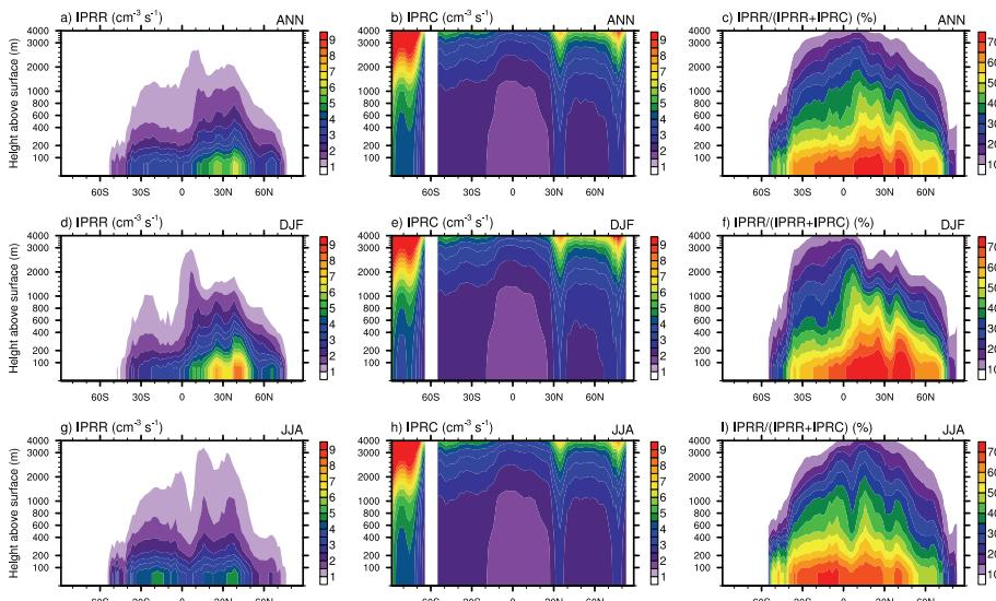
**Fig. 12.** Left column: simulated zonal mean ionization rate over the continents caused by the radioactive decay of radon and its progeny (IPRR, unit:  $\text{cm}^{-3} \text{s}^{-1}$ ); Middle column: as in the left column but caused by galactic cosmic rays (IPRC, unit:  $\text{cm}^{-3} \text{s}^{-1}$ ); Right column: the contribution of radon and its progeny to the total (IPRR + IPRC) ionization rate. All panels correspond to the simulation performed with the merged emission map.
