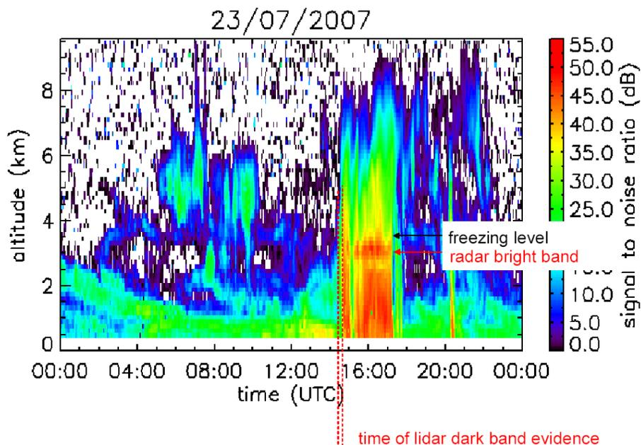
**Fig. 2.** Time evolution of radar reflectivity at 1.29 GHz from 00:00 UTC to 24:00 UTC on 23 July 2007 as measured by the clear air wind profiler. Arrows indicate the location of the freezing level and the radar bright band.
