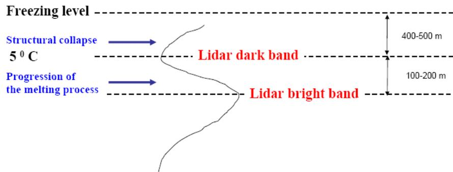
**Fig. 12.** Simplified schematic representation of the the lidar dark and bright band.
