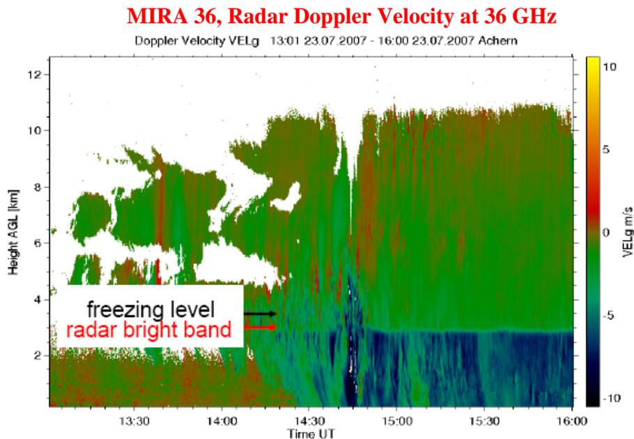
**Fig. 6.** Time evolution of hydrometeors vertical velocity from 13:00 UTC to 16:00 UTC on 23 July 2007 as measured by MIRA 36.
