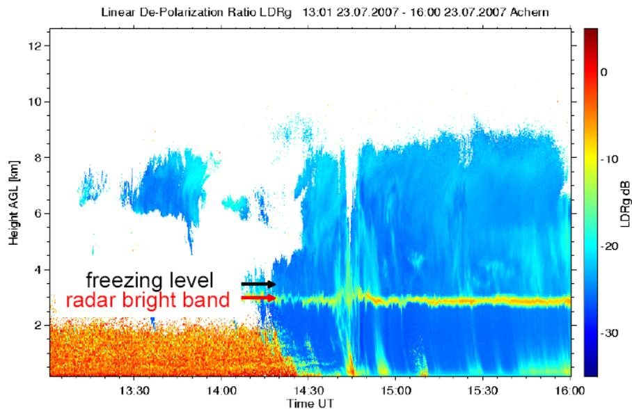
**Fig. 5.** Time evolution of the linear depolarization ratio at 36 GHz from 13:00 UTC to 16:00 UTC on 23 July 2007 as measured by MIRA 36.
