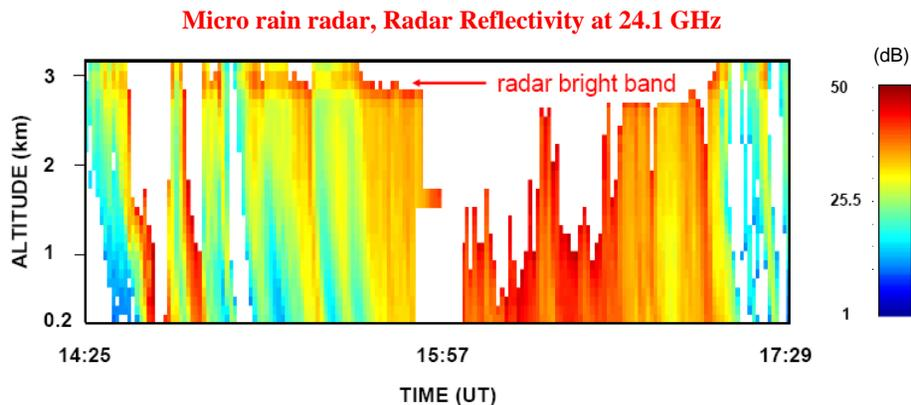
**Fig. 4.** Time evolution of radar reflectivity at 24.1 GHz from 14:25 UTC to 17:29 UTC on 23 July 2007 as measured by the micro rain radar. The red arrow indicates the location of the radar bright band.
