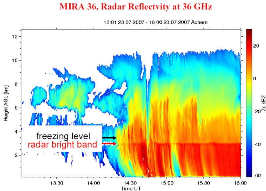
**Fig. 3.** Time evolution of radar reflectivity at 36 GHz from 13:00 UTC to 16:00 UTC on 23 July 2007 as measured by MIRA 36. Arrows indicate the location of the freezing level and the radar bright band.
