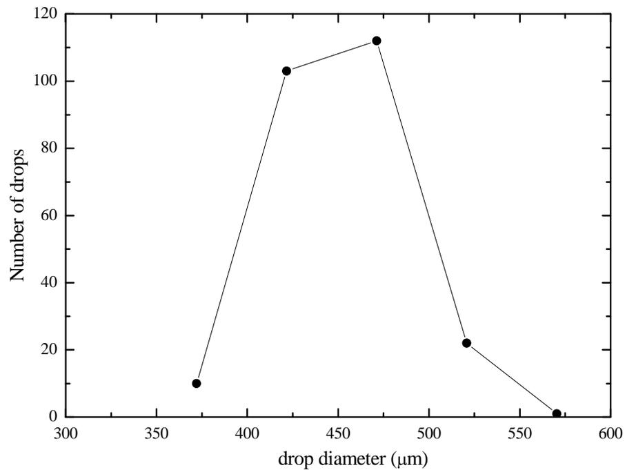
**Fig. 18.** Precipitating particle size distribution as obtained from the time series of the disdrometer measurements at ground level in Supersite *R*.
