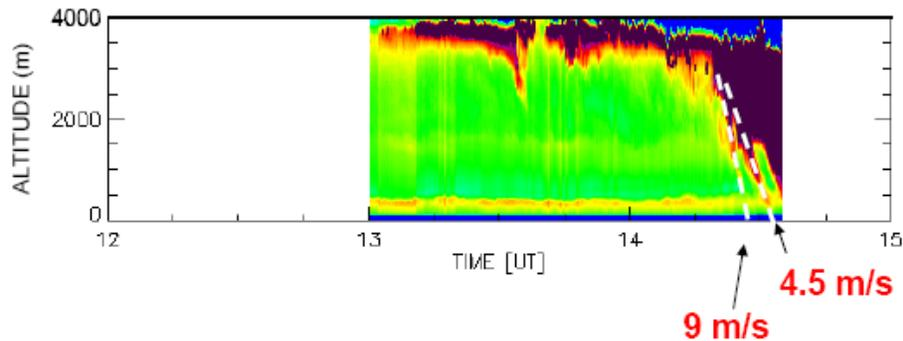
**Fig. 8.** Time evolution of the particle backscatter ratio at 1064 nm from 13:00 UTC to 14:35 UTC on 23 July 2007 as measured by the Raman Lidar system BASIL. In the figure the precipitating hydrometeors with different fall velocities appear as different particle streams with different slopes.
