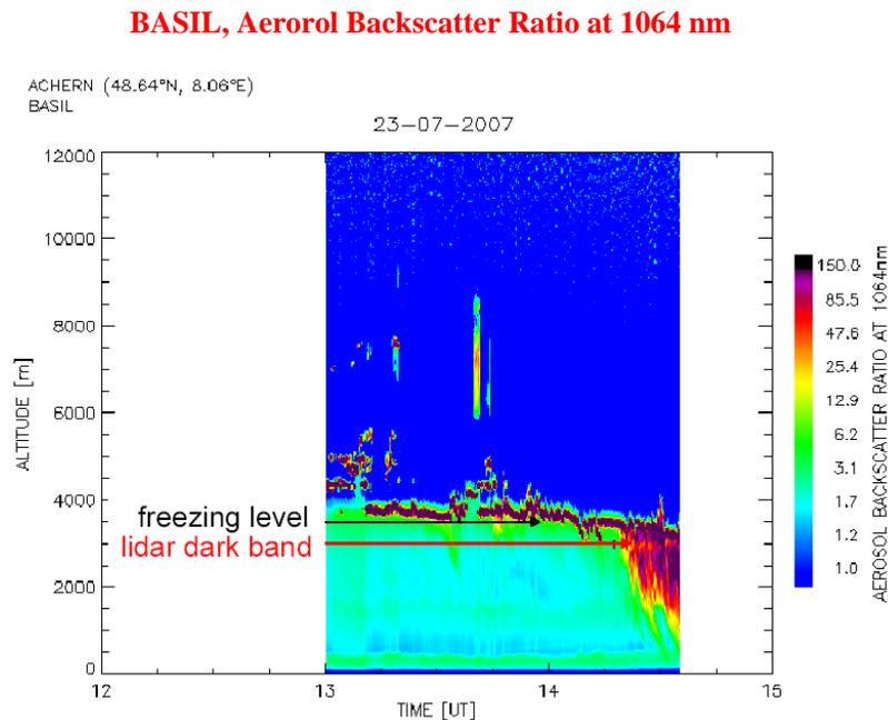
**Fig. 1.** Time evolution of the particle backscatter ratio at 1064 nm from 13:00 UTC to 14:35 UTC on 23 July 2007 as measured by the Raman Lidar system BASIL. Arrows highlight the location of the freezing level and the lidar dark band.
