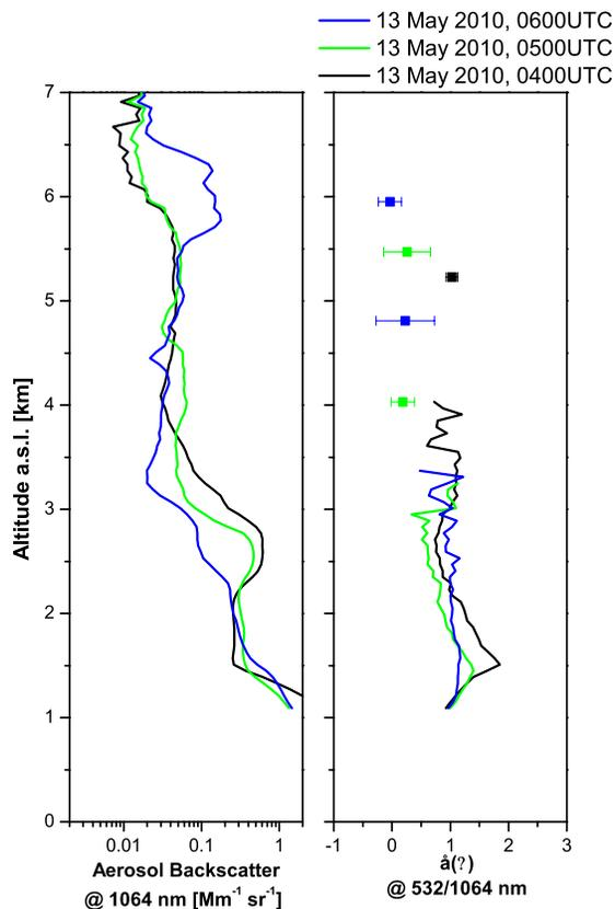
**Fig. 5.** Profiles of the aerosol backscatter at 1064 nm and of the backscatter related Ångström exponent at 532/1064 nm measured on 13 May, at 04:00, 05:00 and 06:00 UTC. Mean values are reported as squares for backscatter related Ångström exponent at altitude levels where corresponding profile is highly noisy. Error bars report the standard errors for the mean values.
