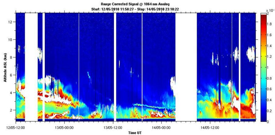
**Fig. 1.** Temporal evolution of range corrected lidar signal measured at 1064 nm in the 12–14 May period by PEARL at CIAO. The vertical and temporal resolutions are respectively 7.5 m and 30 s.
