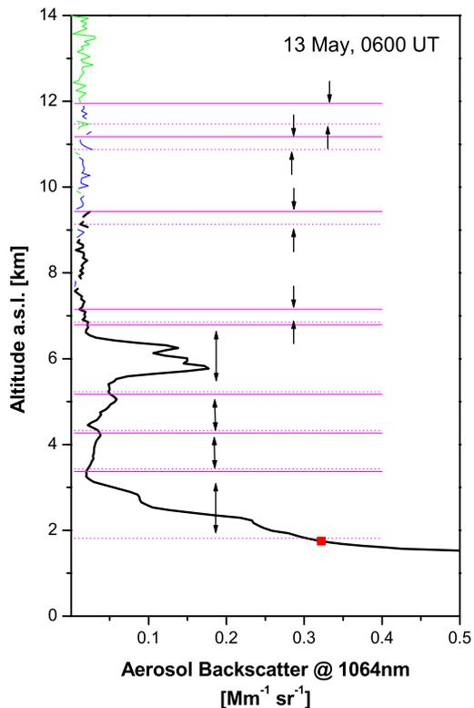
**Fig. 2.** Example of single profile particle layer identification as performed on the aerosol backscatter profile at 1064 nm measured on 13 May, at 05:30–06:30 UTC. Horizontal dotted and solid lines indicate the base and top of the identified layers, respectively. Red square indicates the PBL top height. Region with relative errors between 30–50% are reported in blue and those with relative error exceeding 50% in green.
