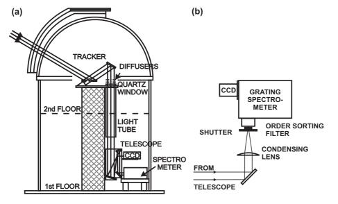
**Fig. 1.** Schematic of the instrument light path. **(a)** Light is collected by the primary of the heliostat (tracker), reflected down to the telescope on the first floor which conditions it to a 7 cm diameter collimated beam. **(b)** The light is then reflected to a condensing lens, past a shutter, order-sorting filter, and then into the spectrometer, recorded by a CCD.
